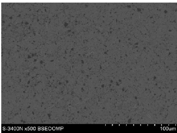
Fig. 6. Microstructure of Al-SiC+C composite, SEM
