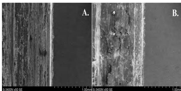
Fig. 7. Surfaces area after wear in Al-Al<sub>2</sub>O<sub>3</sub>+C (A.) and Al-SiC+C (B.) composite, SEM
