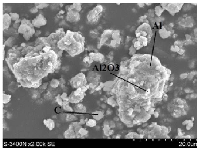
Fig. 3. Composite powder of  $\text{Al}-\text{Al}_2\text{O}_3+\text{C}$ , SEM
