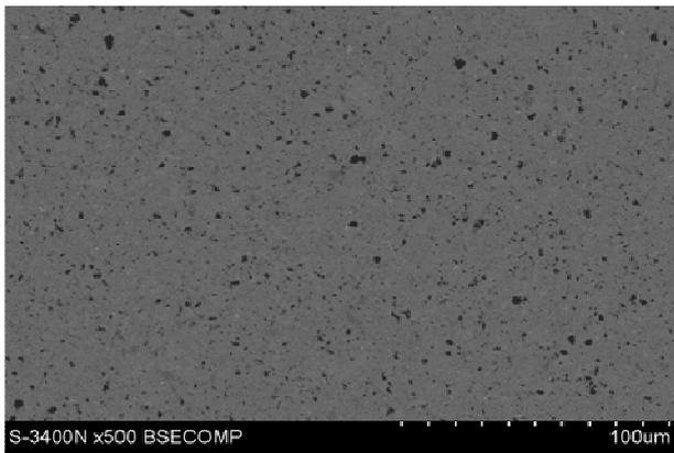
Fig. 5. Microstructure of Al-Al<sub>2</sub>O<sub>3</sub>+C composite, SEM
