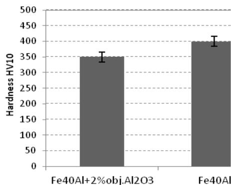
Fig. 6. Hardness for selected technological options
