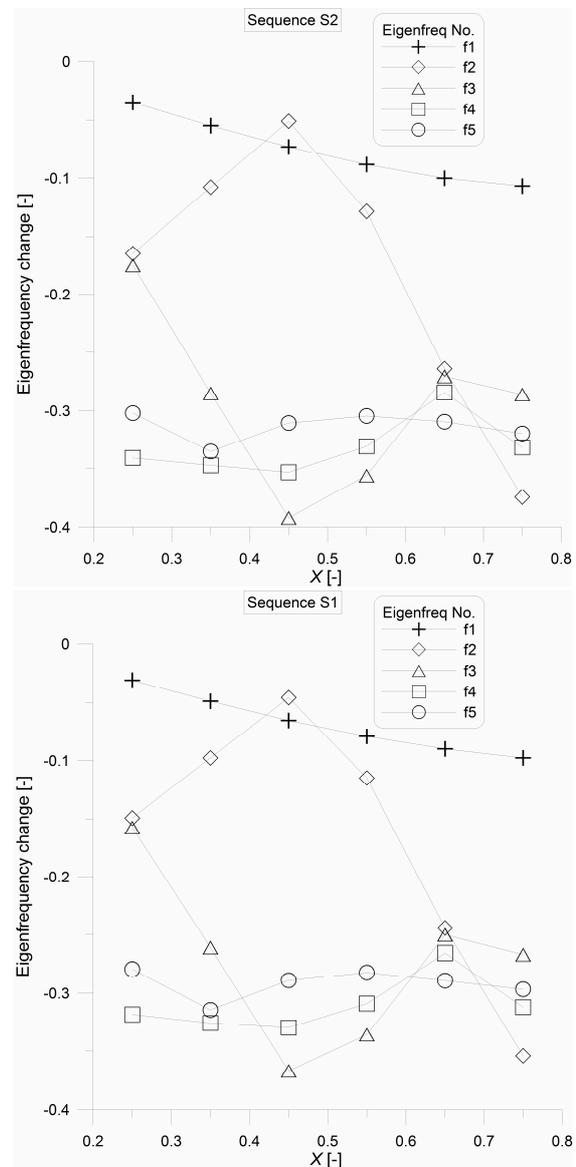
Fig. 3. Influence of half-length delamination on eigenfrequencies of composite cantilever beam
