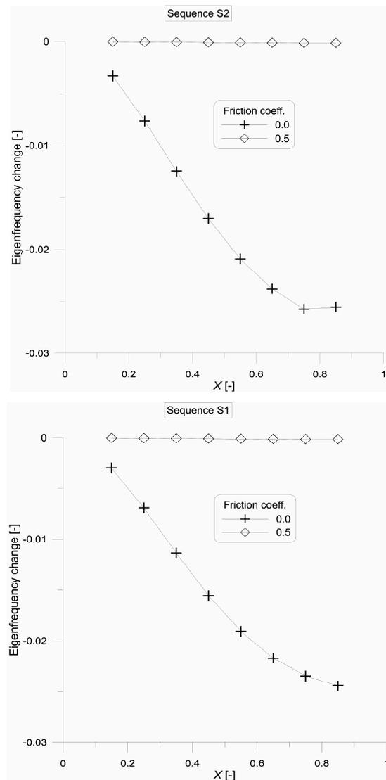
Fig. 7. Relative drop of first eigenfrequency ( $f_1$ ) of composite cantilever beam when friction is taken into account
