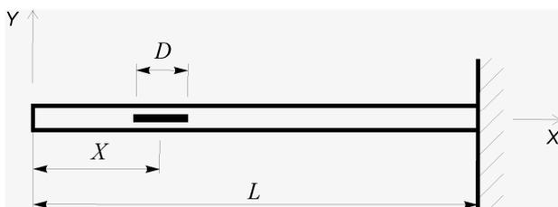
Fig. 1. Delaminated composite cantilever beam model used in numerical simulations
