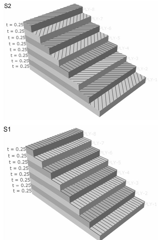
Fig. 2. Ply sequences S1 and S2 of considered FE beam models
