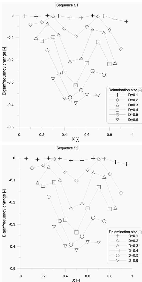
Fig. 6. Relative drop of third eigenfrequency ( $f_3$ ) of composite cantilever beam
