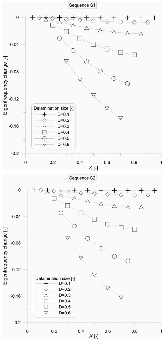
Fig. 4. Relative change of first eigenfrequency ( $f_1$ ) of composite cantilever beam
