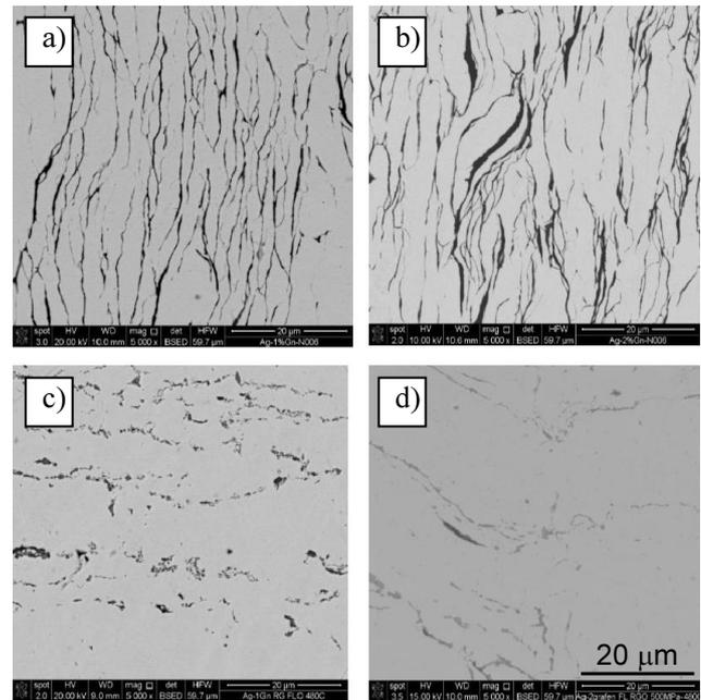
Fig. 4. SEM micrographs of silver matrix composites hot pressed in vacuum containing: a) 1% N006 graphene platelets, b) 2% FLRGO graphene, c) 1% FLRGO graphene, d) 2% FLRGO graphene
