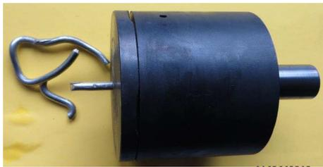
Fig. 3. Die made from heat resistant steel with carbide plunger used for extrusion of Ag based 2% FLRGO graphene platelet composite
