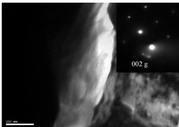
Fig. 9. TEM micrograph of hot pressed and extruded silver based composite and electron diffraction pattern from the area of micrograph shown as an insert
