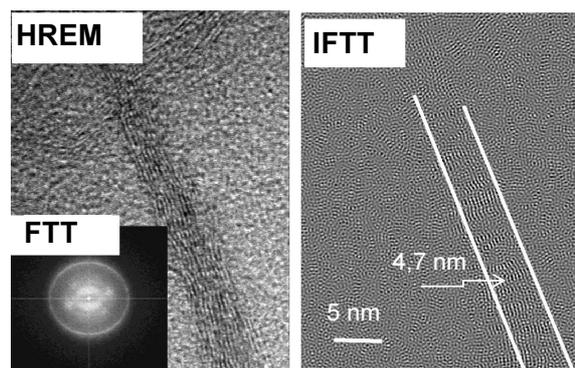
Fig. 2. HRTEM micrograph of graphene platelet with 002 plane oriented parallel to electron beam. In lower corner its Fourier transform (FFT) showing diffused ring from 002 graphite platelet plane and on right side inverse Fourier transform (IFFT) showing fringes from 002 plane in graphene platelet of thickness 4.7 nm in better contrast showing slight misorientation of platelet fragments
