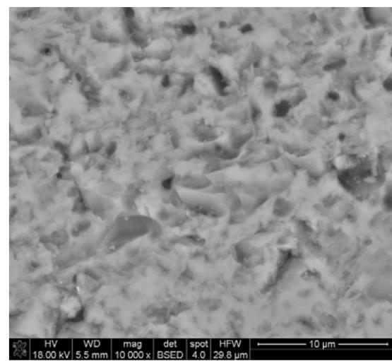
Fig. 5. SEM image of worn SC sample surface after Miller Test
