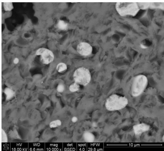
Fig. 6. SEM image of worn SCTB sample surface after Miller Test
