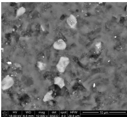
Fig. 2. SEM image of worn SCTB sample surface after Dry Sand Test
