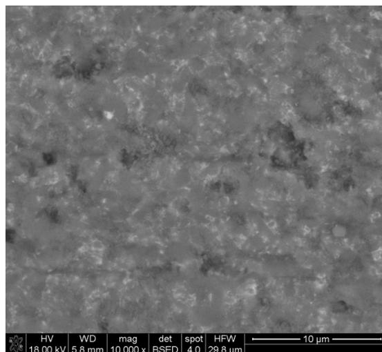
Fig. 8. SEM image of worn SNSC sample surface after Miller Test
