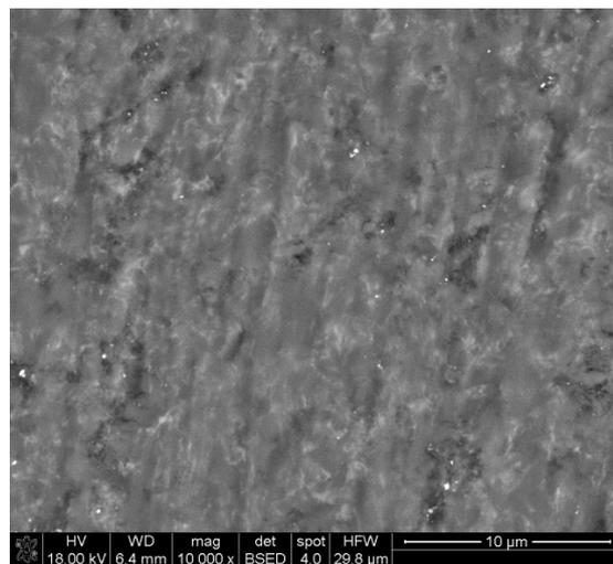
Fig. 3. SEM image of worn SN sample surface after Dry Sand Test
