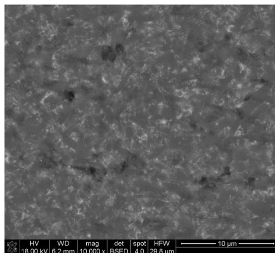
Fig. 4. SEM image of worn SNSC sample surface after Dry Sand Test
