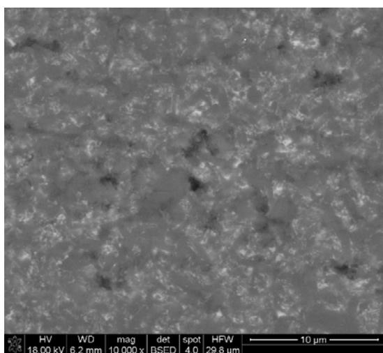
Fig. 7. SEM image of worn SN sample surface after Miller Test Test
