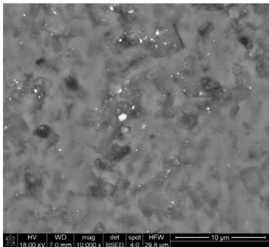
Fig. 1. SEM image of worn SC sample surface after Dry Sand Test
