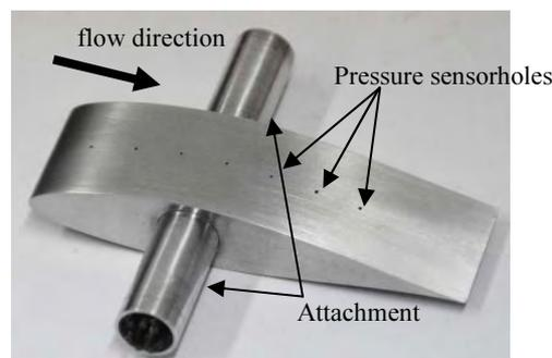
Fig. 1. Rigid NACA 64-418 profile made of aluminum
