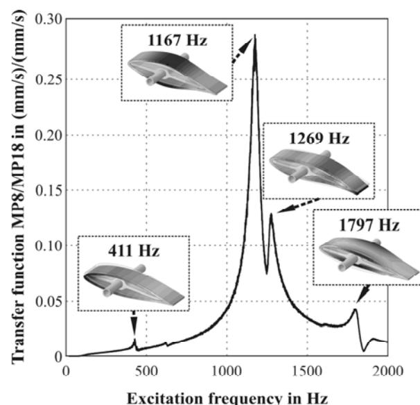
Fig. 6. Identified eigenfrequencies and eigenforms of analysed active aerofoil profile
