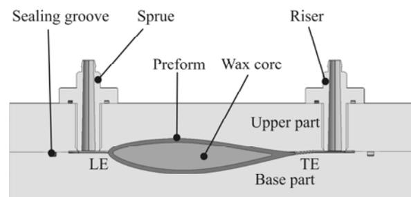
Fig. 4. RTM tool for manufacturing NACA aerofoil (LE - leading edge; TE - trailing edge)
