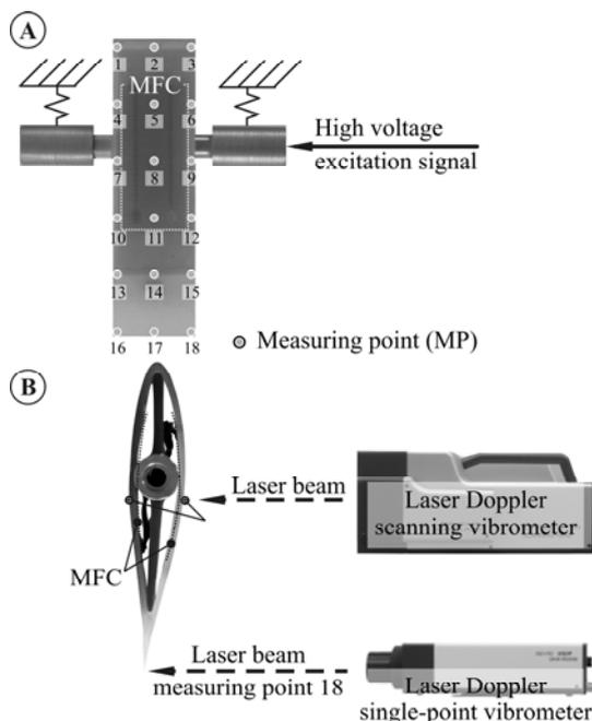
Fig. 5. Experimental set-up used to determine of active aerofoil dynamical properties with marked positions of measurement points and applied MFCs. A - front view, B - side view
