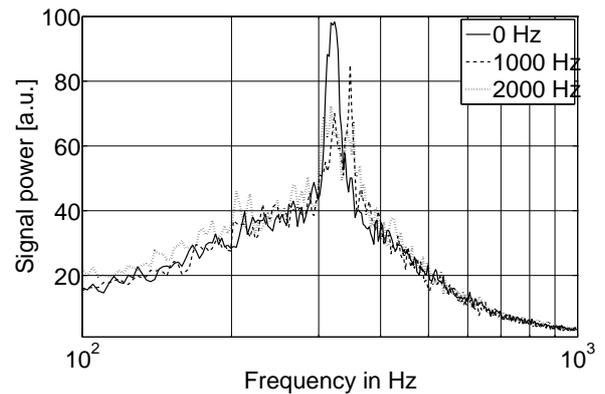
Fig. 8. Amplitude spectrum of measured signal at different excitation/actuator frequencies. Position of hot wire probe is 10 mm downstream of the profile at middle of test channel cross section
