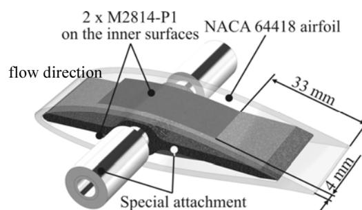
Fig. 2. NACA aerofoil in FRP design with special attachment
