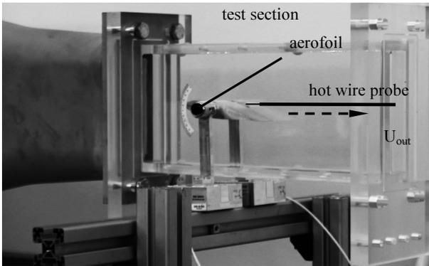
Fig. 7. Test section with installed aerofoil profile and sketch of hot wire probe
