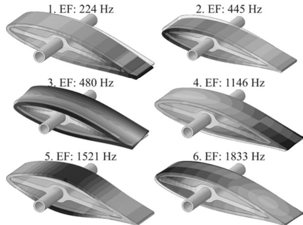
Fig. 3. First six eigenmodes of NACA aerofoil calculated using FEM
