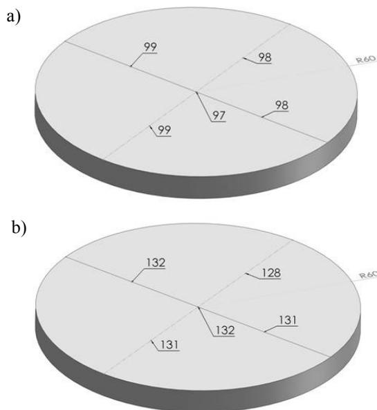
Fig. 9. Hardness comparison for AlZn5.5MgCu alloy (a) and AlZn5.5MgCu + cenospheres composite (b)
