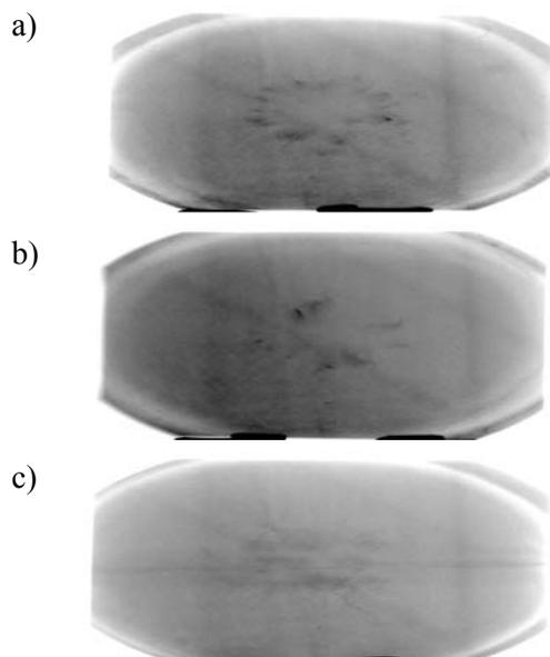
Fig. 6a-c. Result of ALFA composites X-ray inspection
