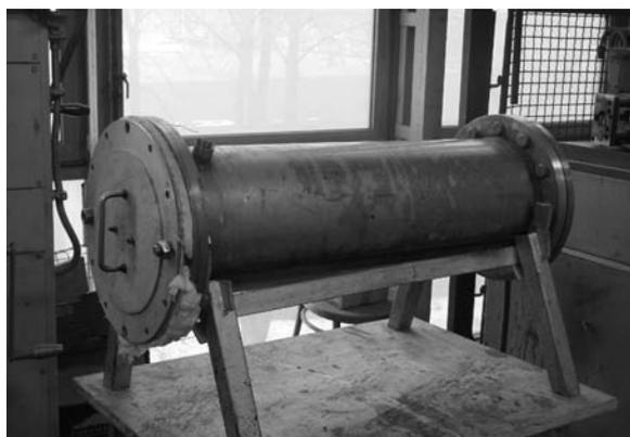
Fig. 4. View of heat treatment furnace for pre-heating preforms
