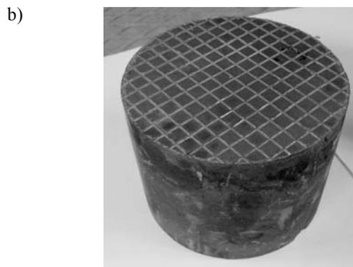
Fig. 5. a) View of die interior on stand for pressure infiltration, b) composite casting
