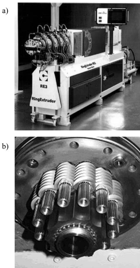
Fig. 1. a) Ring Extruder is designed for more elongational mixing vs. shear mixing for more efficient compounding, b) twelve co-rotating, fully intermeshing, self-wiping screws rotate around their own axes and do not rotate around stationary core
