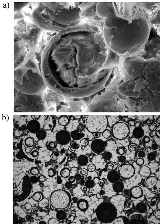
Fig. 8. a) SEM analysis of cenospheres, b) microstructure of syntactic foam (AlZn5.5MgCu + cenospheres)
