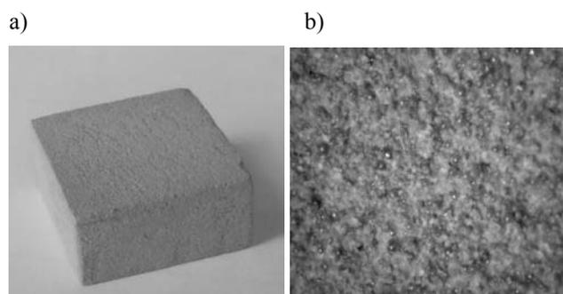
Fig. 2. a) Ceramic preform made by Century, b) preform surface
