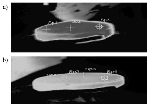
Fig. 7. Thermal analysis of infiltration process - temperature distribution in preform before infiltration; a) variant: AlZn5.5MgCu + ceno, Sp1 - 660°C, Sp2 - 667°C, Sp3 - 683°C, b) variant: AlZn5.5MgCu+ceno, Sp1 - 609°C, CSp2 - 625°C, Sp3 - 642°C, Sp4 - 646°C
