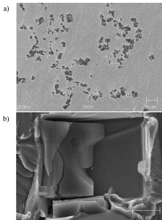
Fig. 2. Microstructure of Ni<sub>3</sub>Al/TiC composite, 500x, (a), and scanning image of Ni<sub>3</sub>Al/TiC composite fracture, 5000x (b)
