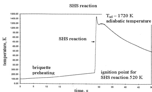
Fig. 1. Temperature - time relationship in standard SHS method during synthesis of  $TiB_2$
