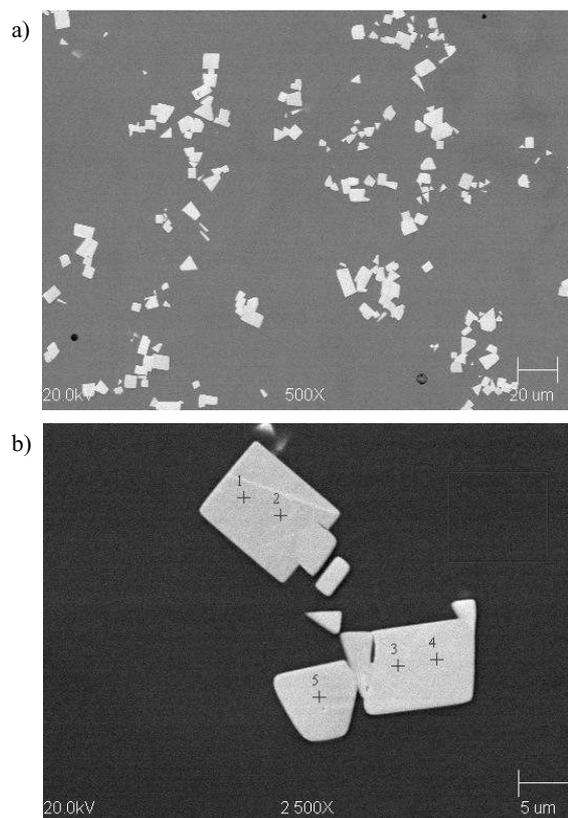
Fig. 6. Microstructure of  $Ni_3Al/TaC$  composite, 500x, (a), image with marked points of chemical analysis, 2500x (b).
