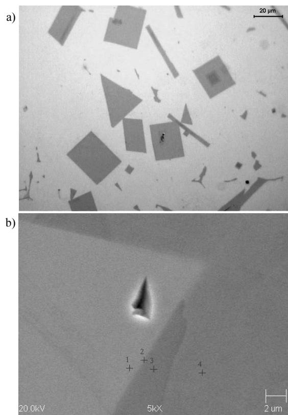
Fig. 4. Microstructure of Ni<sub>3</sub>Al/ZrC composite, 500x, (a), scanning topographic image of Ni<sub>3</sub>Al/ZrC composite, 5000x (b)
