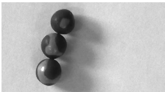
Fig. 2. Incorrect selection of grinding parameters - permanent deposition of Al (darker area) on surface of grinding media (lighter area)
