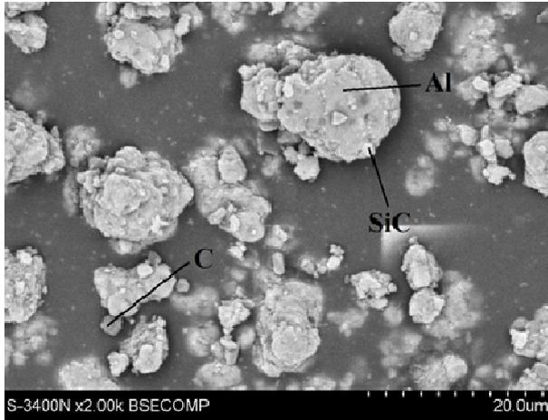
Fig. 4. Al-SiC+C composite powder, SEM
