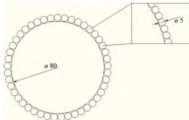
Fig. 1. Layer of ceramic particles with  $5\ \mu m$  diameter on surface of matrix particles with  $80\ \mu m$  diameter
