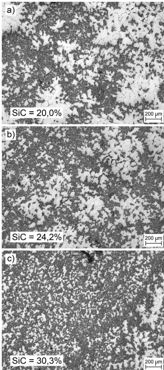
Fig. 7. Microstructure of  $\phi 13$  mm casting obtained with centrifugal force: a) upper area, b) central area, c) bottom area
