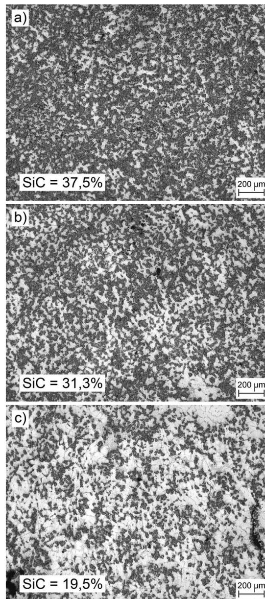
Fig. 5. Microstructure of  $\varnothing 6$  mm casting obtained using centrifugal force: a) upper area, b) central area, c) bottom area
