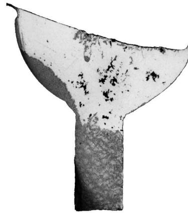
Fig. 8. Micrographs of gating system with visible reinforcement-matrix interface
