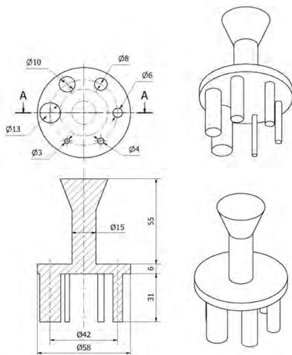
Fig. 1. Diagram of casting model used for tests
