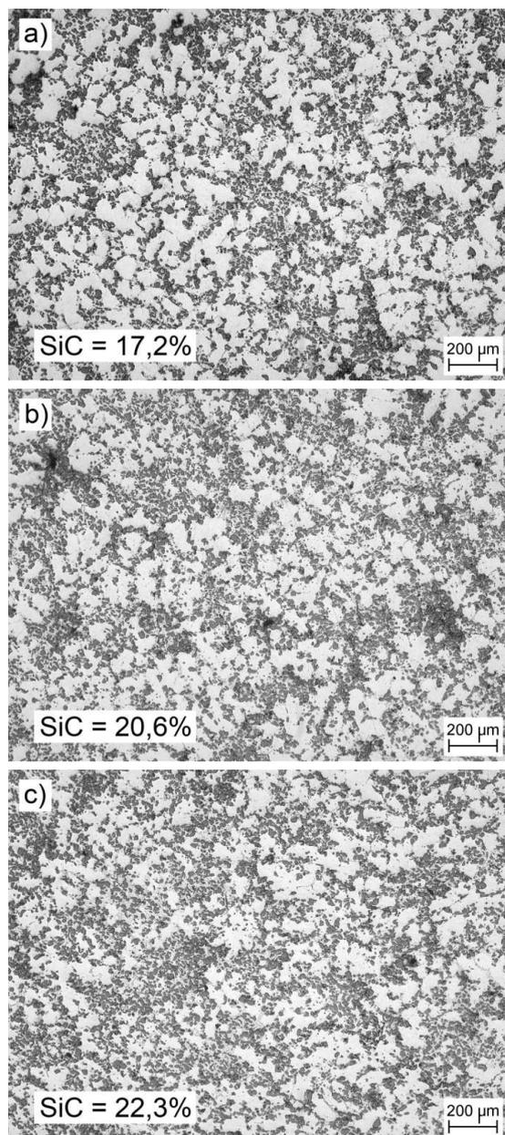
Fig. 4. Microstructure of  $\varnothing 13$  mm casting obtained gravitationally: a) upper area, b) central area, c) bottom area
