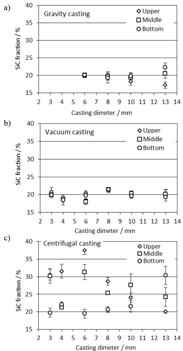
Fig. 3. Distribution of SiC particles depending on diameter of casting for molds filled: a) gravitationally, b) with subatmospheric pressure, c) centrifugally
