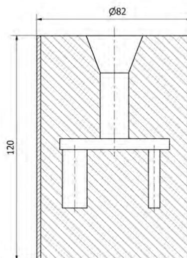
Fig. 2. Diagram of casting mold section
