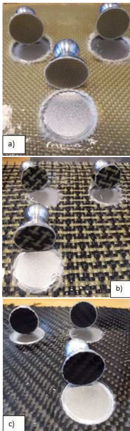
Fig. 6. Epoxy coating after pull-off test: a) with aramid fabric, b) with aramid-carbon fabric, c) with carbon fabric
