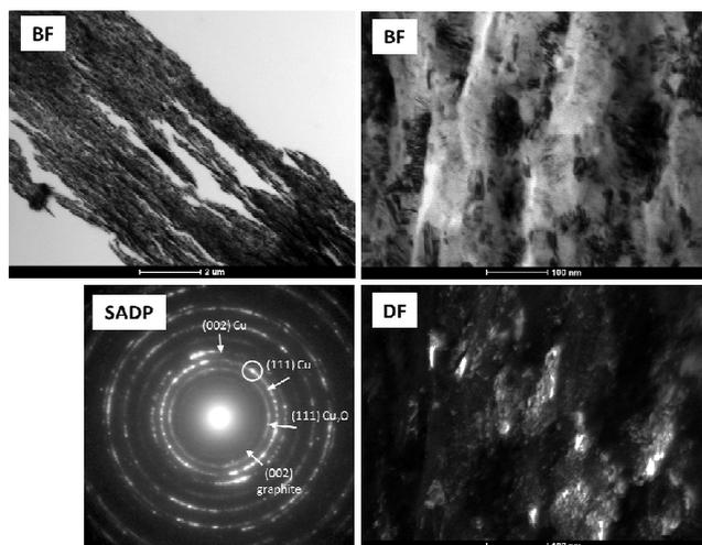
Fig. 6. TEM/BF micrographs taken at two different magnifications, corresponding SADP and DF micrograph of Cu+3%CNT powder mixture after 4 hours of milling
