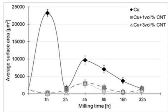
Fig. 4. Mean surface area of Cu+CNT powder mixture particles after various milling times. Untypical scale of milling time (neither linear, nor logarithmic) was chosen to make it easier for the reader to follow particle surface area changes
