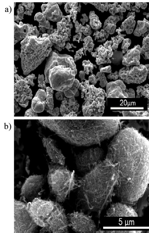
Fig. 1. SEM/SE micrographs of as-supplied copper powder (a) and CNTs (b)
