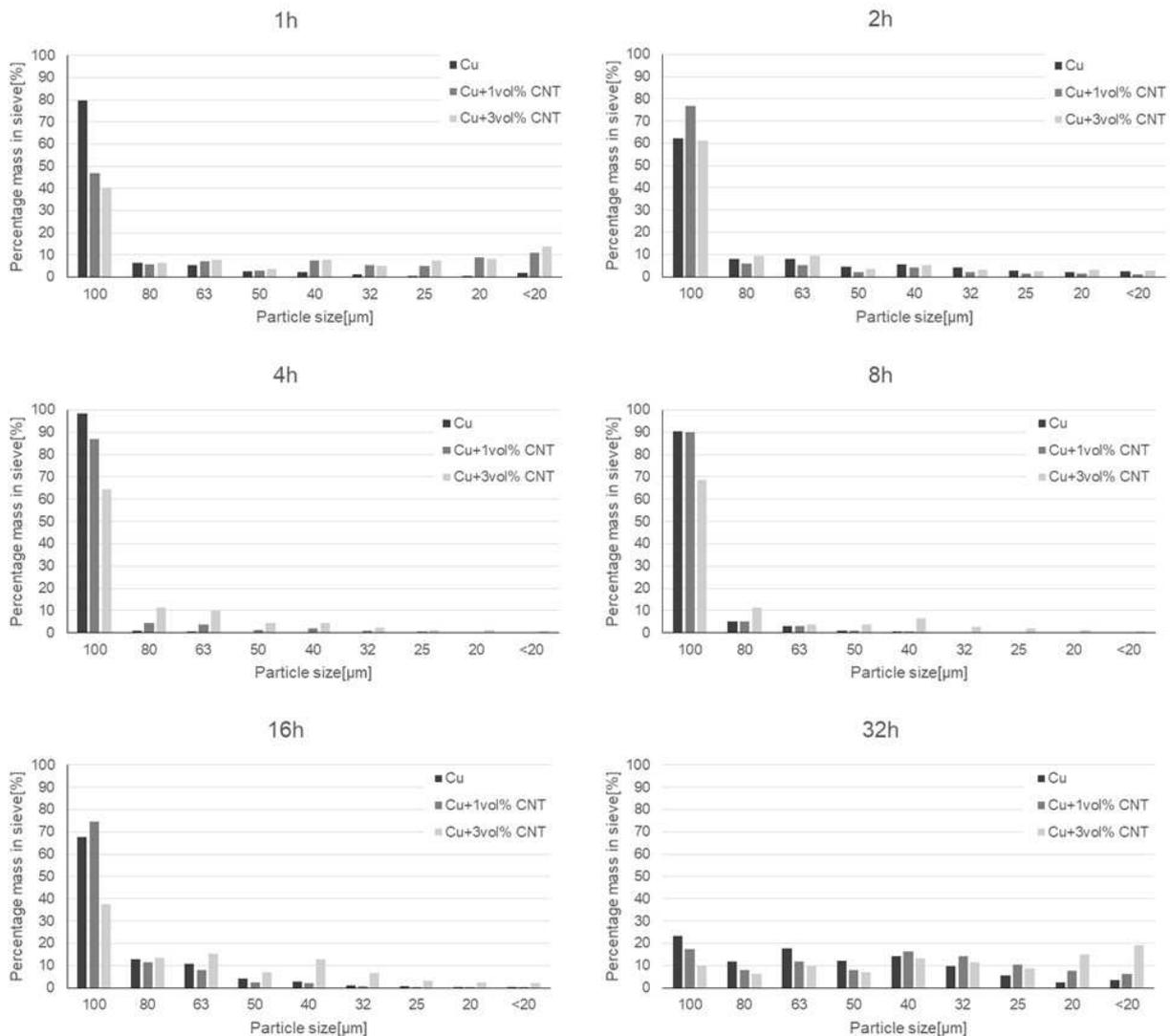
Fig. 5. Histograms of Cu+CNT powder mixture particle size (1 and 3 vol.% CNTs) obtained by sieve analysis
