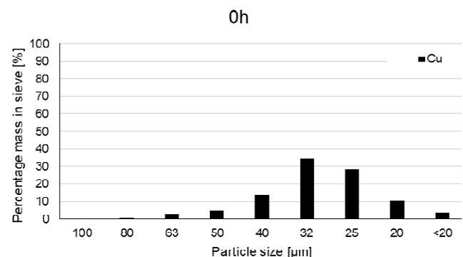
Fig. 2. Histogram of particle size of as-supplied copper powder obtained by sieve analysis
