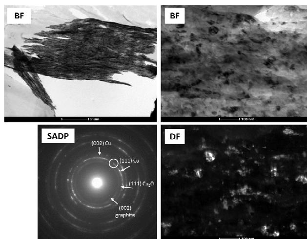
Fig. 7. Set of TEM micrographs of microstructures of Cu+3%CNT powder mixture after 8 hours of milling
