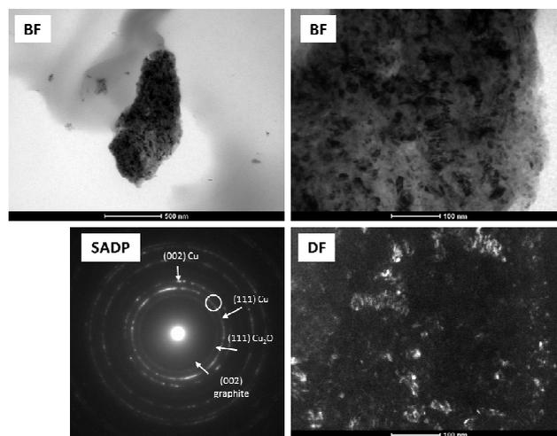
Fig. 8. Set of TEM micrographs of microstructures of Cu+3%CNT powder mixture after 32 hours of milling
