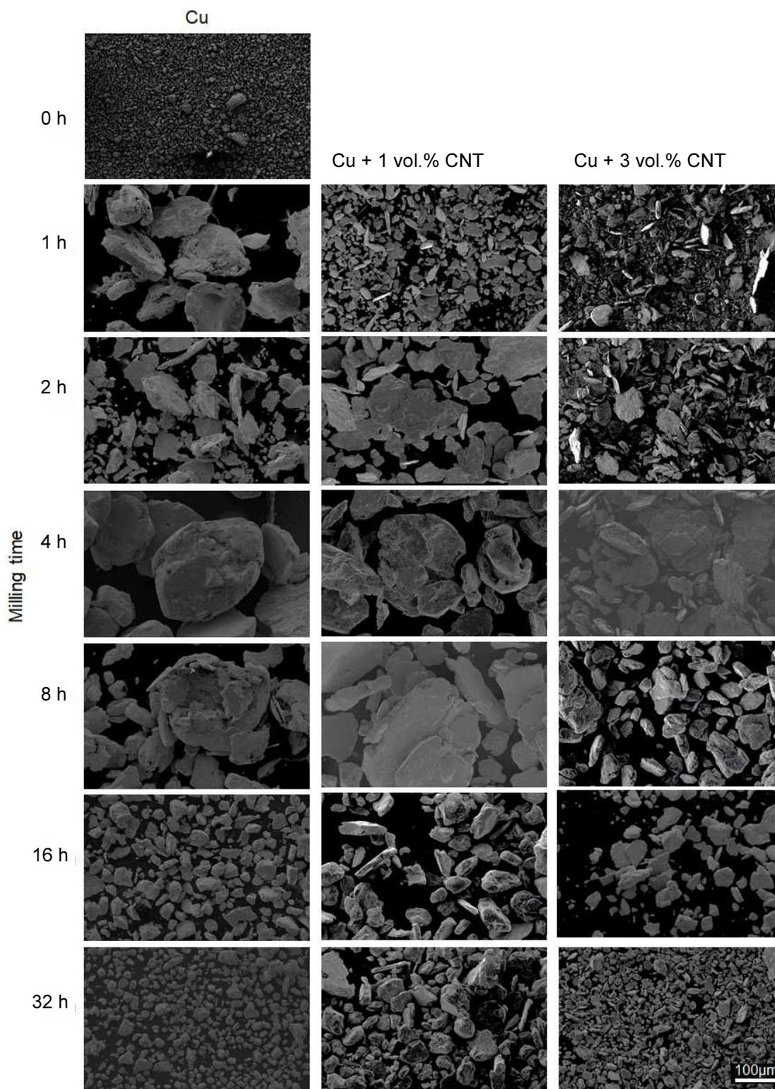
Fig. 3. SEM/SE micrographs of copper powder with addition of CNTs after various milling times
