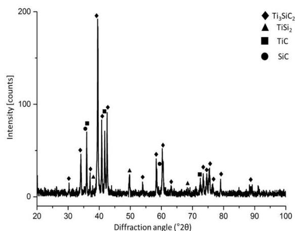
Fig. 4. XRD analysis of manufactured preform
