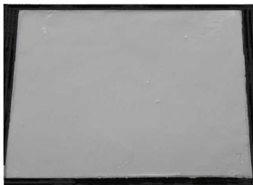
Fig. 1. Sample for thermal conductivity measurements with visible surface defects
