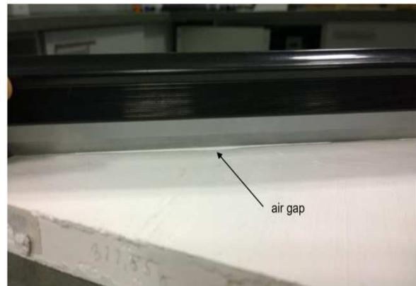
Fig. 5. Air gap between hot plate and sample influencing measurement accuracy
