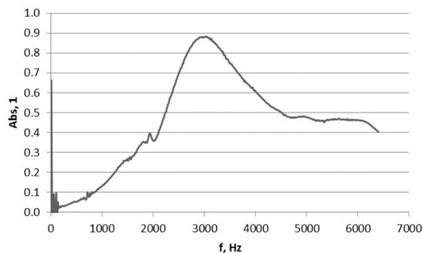
Fig. 7. Sound absorption coefficient of Composite 5 - straw
