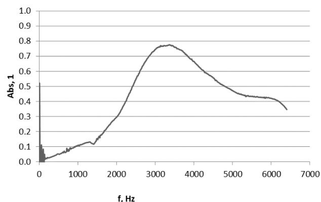
Fig. 4. Sound absorption coefficient of Composite 2 - wooden sawdust
