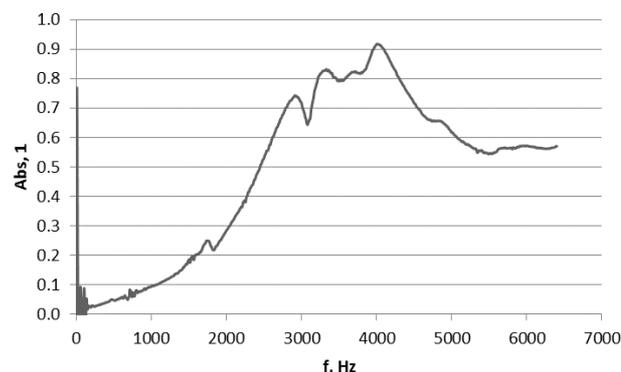
Fig. 3. Sound absorption coefficient of Composite 1 - wood flakes
