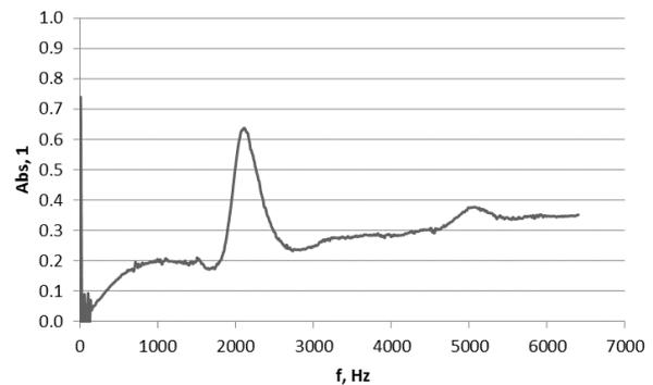
Fig. 9. Sound absorption coefficient of Composite 7 - flax fibers
