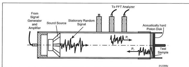
Fig. 2. Set-up with Kundt tube schematic diagram of impedance tube (technical documentation, Brüel&Kjaer, Denmark)
