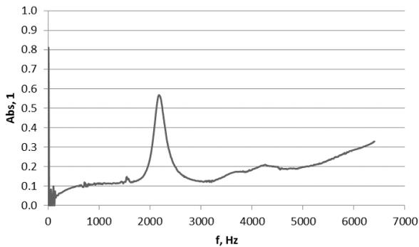
Fig. 5. Sound absorption coefficient of Composite 3 - cork
