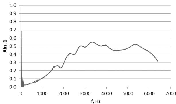
Fig. 6. Sound absorption coefficient of Composite 4 - paper
