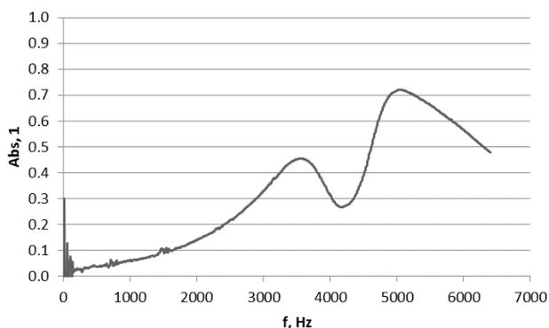
Fig. 8. Sound absorption coefficient of Composite 6 - feather calamus
