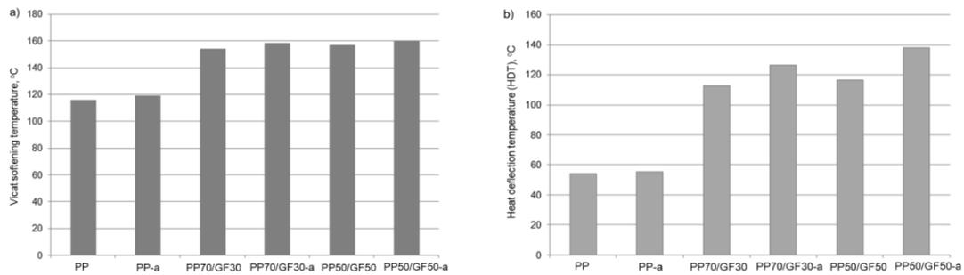
Fig. 6. Thermal properties of tested samples: a) Vicat softening temperature, b) heat deflection temperature (HDT)
