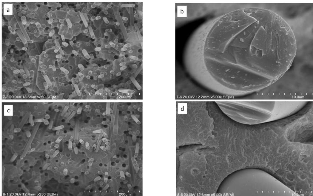
Fig. 8. Fracture microstructure: a) and b) composite PP50/GF50, c) and d) composite PP50/GF50-a (magn. 250 and 5000x)
