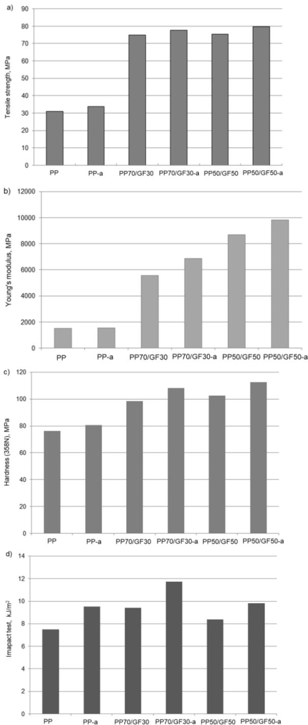
Fig. 5. Mechanical properties of studied composites: a) tensile strength, b) Young's modulus, c) hardness, d) impact test
