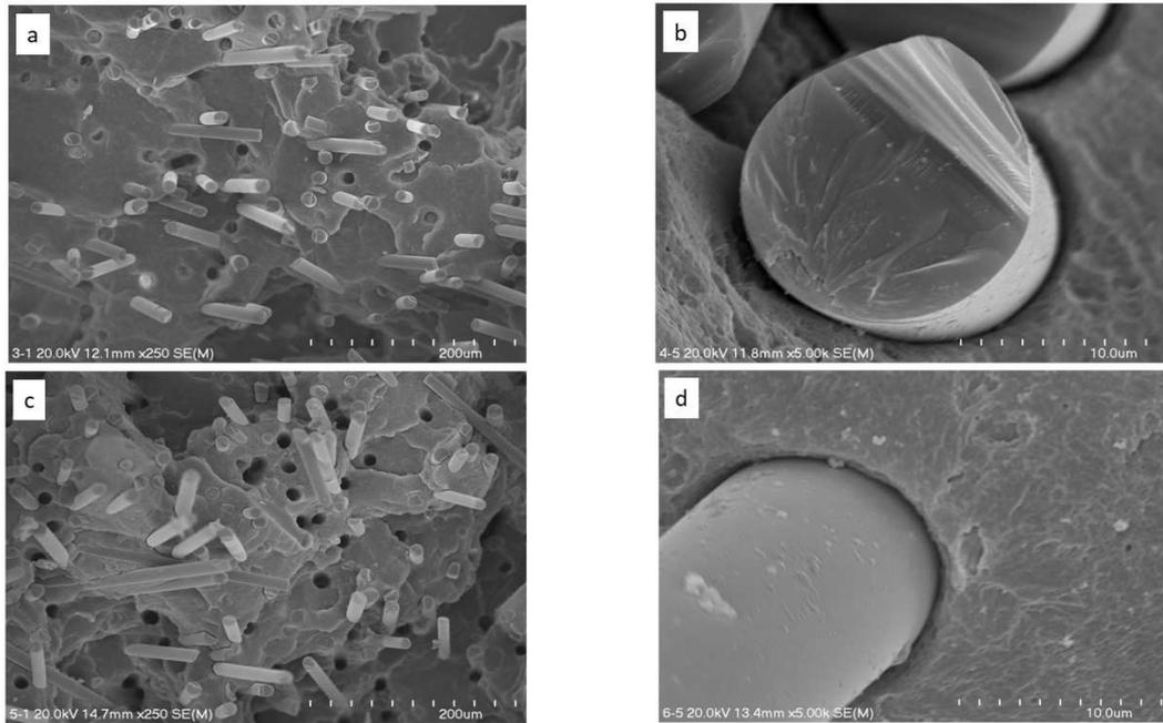
Fig. 7. Fracture microstructure: a) and b) composite PP70/GF30, c) and d) composite PP70/GF30-a (magn. 250 and 5000x)
