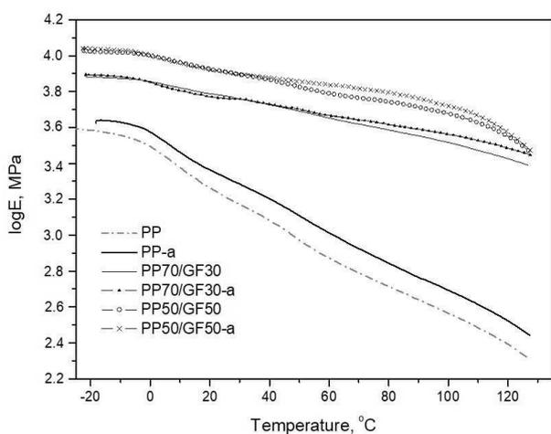
Fig. 2. Dependence of storage modulus ( $\log E'$ ) as function of temperature at frequency of 3 Hz
