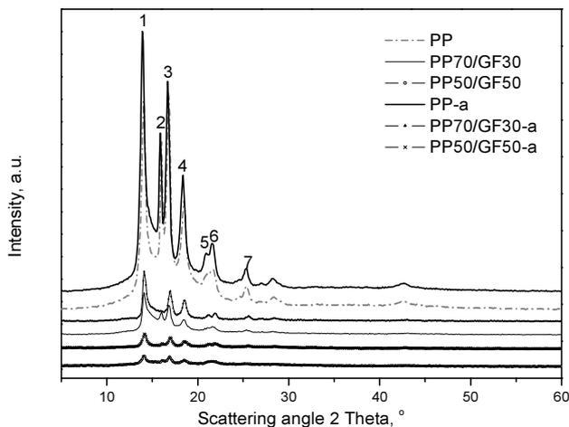
Fig. 1. Diffraction curves for polypropylene and composites
