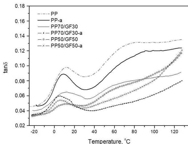
Fig. 3. Dependence of loss tangent coefficient ( $\tan\delta$ ) as function of temperature at frequency of 3 Hz
