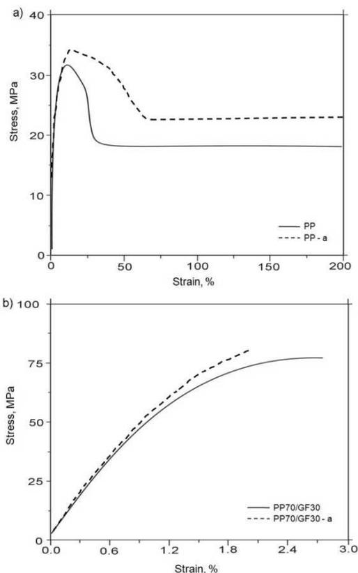
Fig. 4. Relations between stress and strain for tested samples: a) PP. b) composite PP70/GF30
