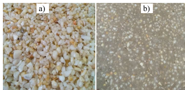
Fig. 4. Surfaces of hardened polymer concrete produced as part of the work: a) only gravel aggregate, b) gravel-sand aggregate
