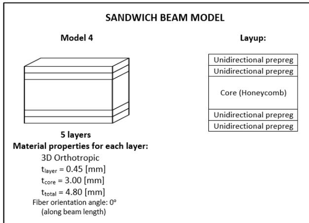
Fig. 13. Parameters of sandwich beam model
