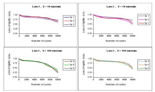
Fig. 9. Loss of rigidity mean curves vs cycles, for given velocities
