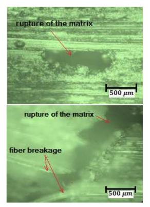
Fig. 7. Fractography of damaged Lam 2 specimen
