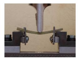
Fig. 3. Three-point bending test
