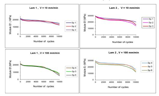
Fig. 8. Flexural modulus mean curves vs cycles, for given velocities
