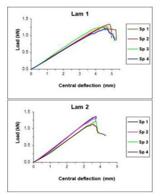
Fig. 4. Load evolution with deflection (Lam 1 and Lam 2)
