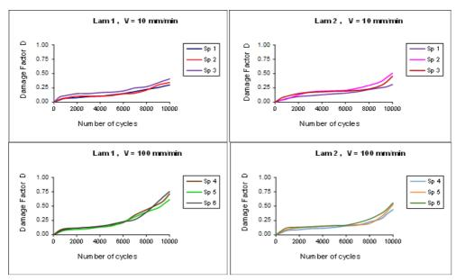
Fig. 10. Damage factor mean curves vs cycles, for given velocities
