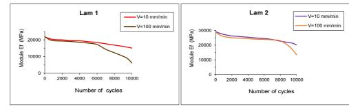
Fig. 11. Effect of testing velocity on fatigue behaviour of laminates
