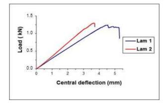
Fig. 5. Mean loading curves vs deflection (Lam 1 and Lam 2)
