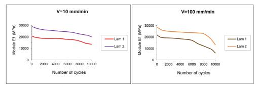
Fig. 12. Fatigue behaviour comparison for selected speeds
