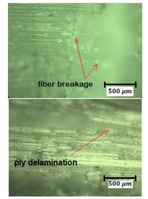
Fig. 6. Fractography of damaged Lam 1 specimen
