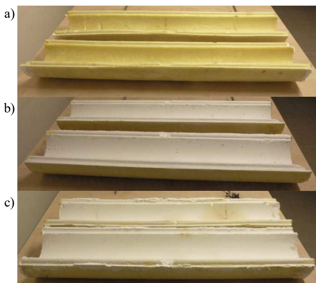
Fig. 1. Shaped insulating material: a) PUR, b) PUR with matrix material coating, c) PUR with composite coating
