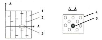
Fig. 3. Unidirectional layer composite: 1 – bundles, 2 – matrix, 3 – crack bundles, 4 – elementary failure volume, 5 – failed
