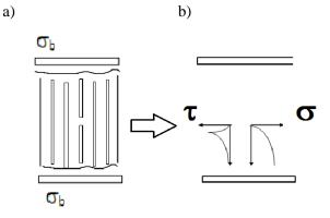
Fig. 4. Critical failure zone: a) failure of bundle, b) diagrams of changes in stresses  $\tau$  and  $\sigma$
