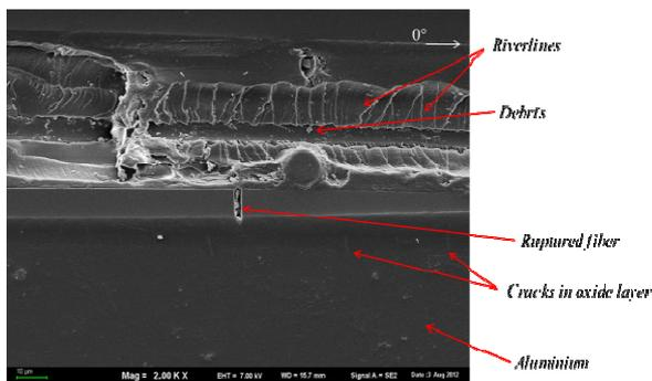
Fig. 8. Cracks and degradation of FML interface, direction [0°], longitudinal section, anodising Cr+P, SEM
