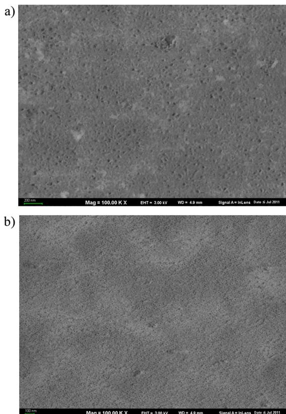
Fig. 6. Anodic oxide layer on aluminium alloy: a) CAA, b) SAA; SEM
