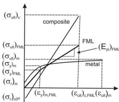
Fig. 3. Schematic uniaxial stress-strain curves for metal, prepreg (composite) and laminate (FML) by [8]; designations in text
