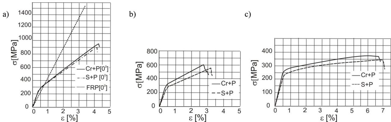
Fig. 4. Typical stress-strain curves for laminates with different fibre orientations and anodising: a)  $[0^\circ]$  Cr+P, S+P, b)  $[0/90^\circ]$  Cr+P, S+P, c)  $[\pm 45^\circ]$  Cr+P, S+P; FRP $[0^\circ]$  - sample of UD glass composite
