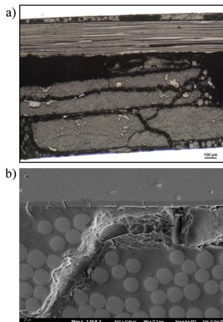
Fig. 10. Degradation of laminate structure with [0/90°] configuration: a) optical microscope, b) SEM; Cr+P anodising
