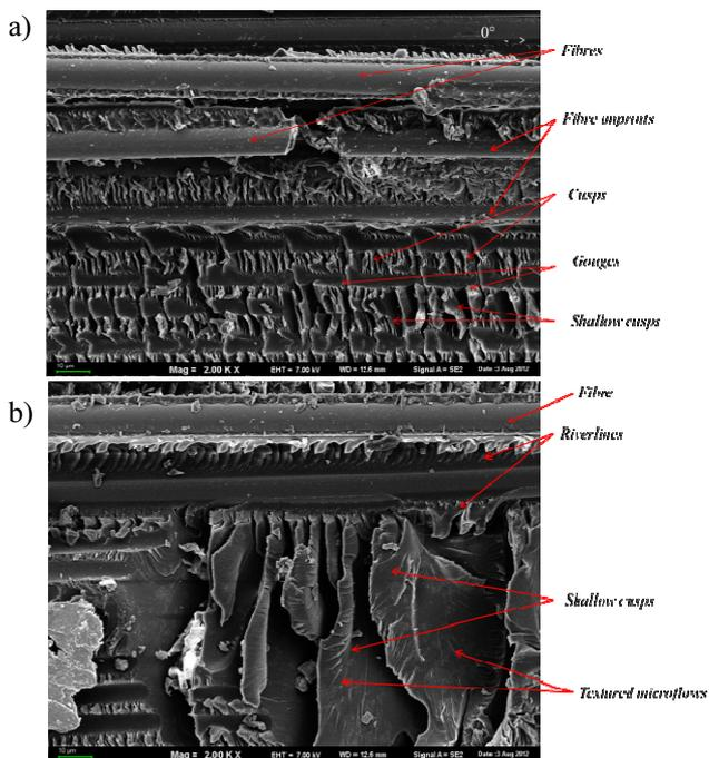
Fig. 9. Aluminium surface morphology after tension test, fibre configuration [0°], anodizing Cr+P; SEM
