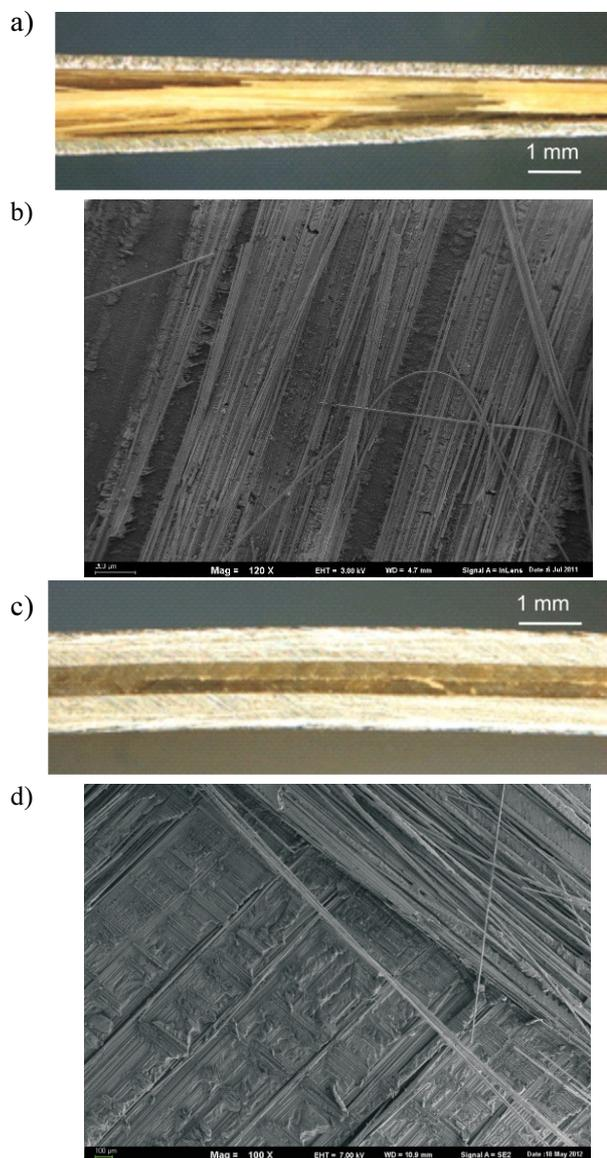
Fig. 7. Degradation of FML sample structure after tensile strength test: a) macrostructure of Al/GFRP $[0^\circ]$ , b) surface of sheet with residual of  $[0^\circ]$  composite, c) macrostructure of Al/GFRP $[\pm 45^\circ]$ , d) surface of sheet with residual of  $[\pm 45^\circ]$  composite; Cr+P anodizing
