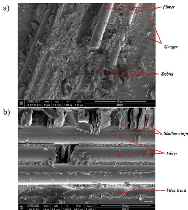
Fig. 11. Aluminium surface morphology after tension tests, S+P anodising, fibre layout [0°]; SEM
