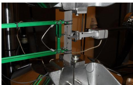
Fig. 2. FML strength properties testing stand
