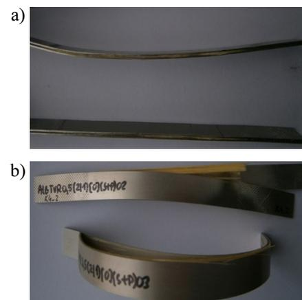
Fig. 5. FML laminate samples after tensile strength test: a) anodising in Cr+P, b) anodising in S+P;  $[0^\circ]$
