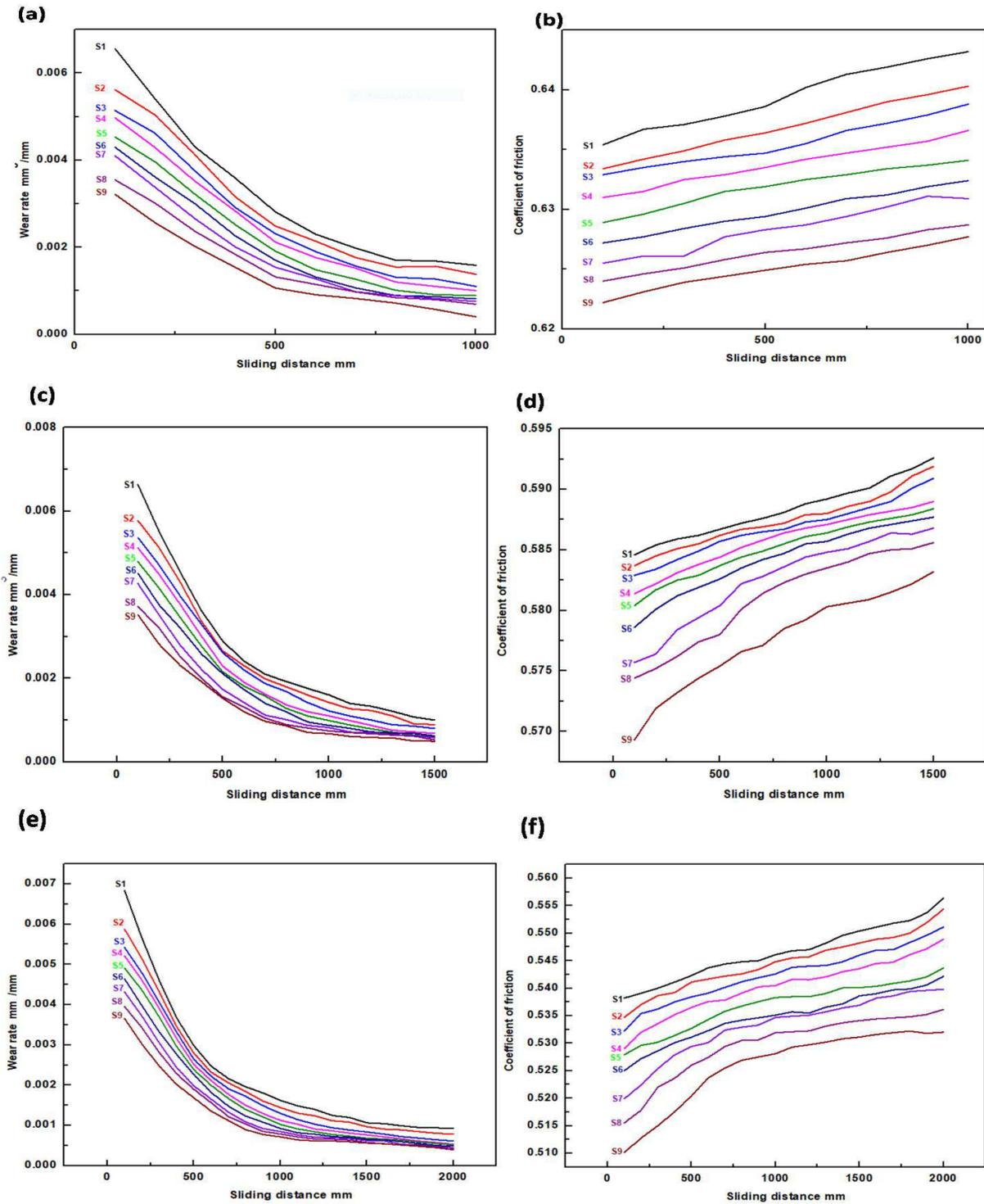
Fig. 6. Variation in wear rate at: a) 20 N, c) 30 N, e) 40 N and coefficient of friction at: b) 20 N, d) 30 N, f) 40 N
