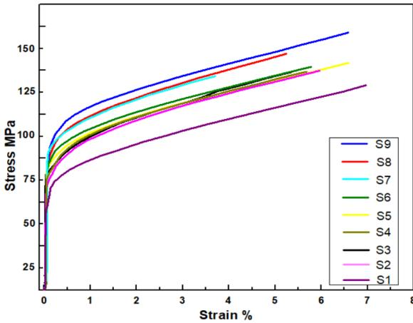
Fig. 3. Stress-strain plot of hybrid composites
