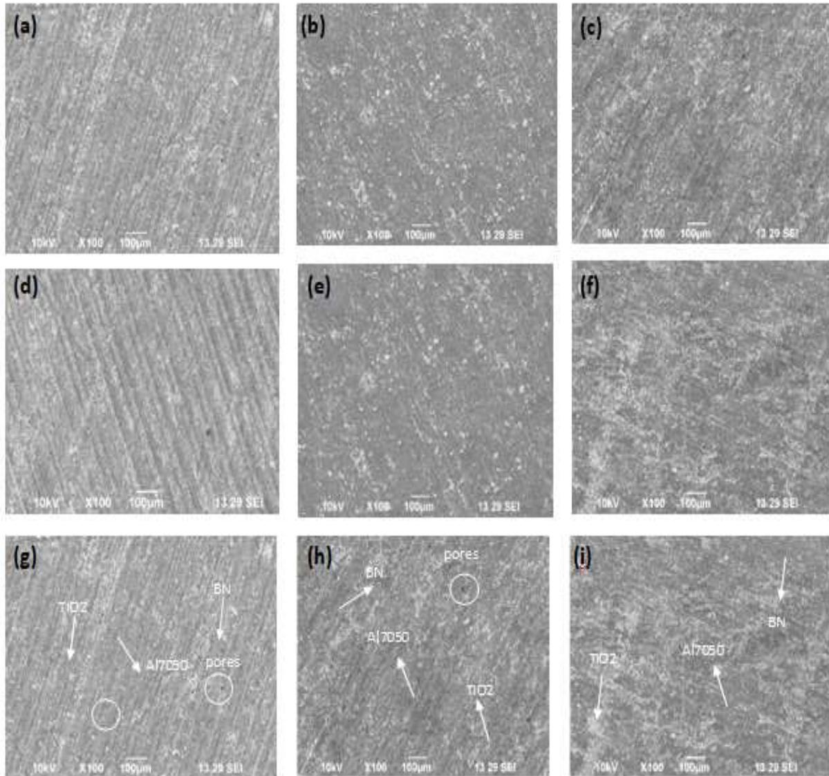
Fig. 2. SEM micrographs of produced composites: a) 1 wt.%, b) 3 wt.%, c) 5 wt.%  $\text{TiO}_2$  at constant 2 wt.% BN, d) 1 wt.%, e) 3 wt.%, f) 5 wt.%  $\text{TiO}_2$  at constant 4 wt.% BN, g) 1 wt.%, h) 3 wt.%, i) 5 wt.%  $\text{TiO}_2$  at constant 6 wt.% BN
