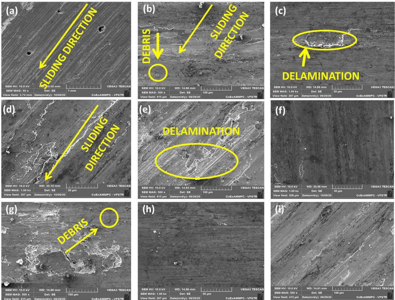
Fig. 8. SEM micrographs showing worn surface of cast hybrid composites with varying percentages of TiO<sub>2</sub> and BN: a) 7050T1B2, b) 7050T3B2, c) 7050T5B2, d) 7050T1B4, e) 7050T3B4, f) 7050T5B4, g) 7050T1B6, h) 7050T3B6, i) 7050T5B6
