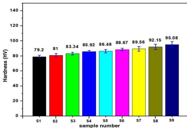
Fig. 4. Hardness of samples with varying weight percentages of TiO<sub>2</sub> and h-BN
