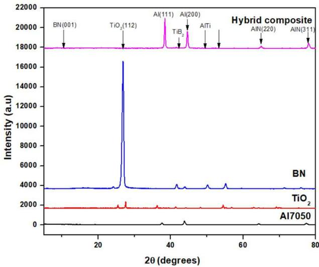
Fig. 7. XRD pattern of Al7050, TiO<sub>2</sub>, h-BN and hybrid composite
