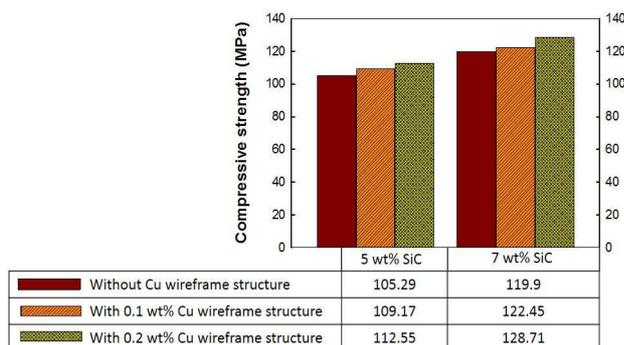
Fig. 3. Comparison of compressive strength [MPa] of composites with different compositions
