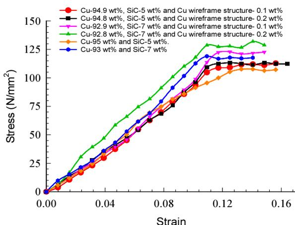
Fig. 4. Stress-strain curve of composites with different composition
