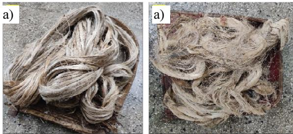
Fig. 1. Natural fibres (a) sisal fibre (SF) and (b) jute fibre (JF)
