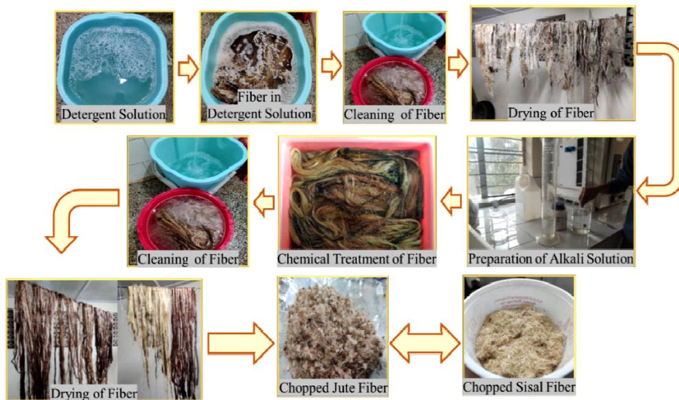
Fig. 2. Processing of chosen natural fibres
