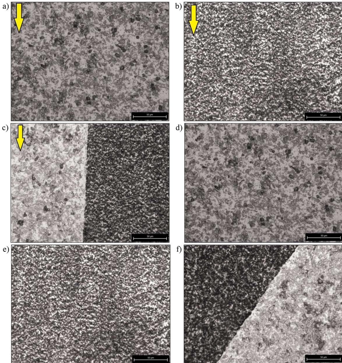
Fig. 7. Bimetallic composite obtained by extrusion at 480°C of components in Al<sub>17</sub>Si<sub>5</sub>Fe<sub>3</sub>Cu<sub>1.1</sub>Mg<sub>0.6</sub>Zr-aluminum sinter. Cross-sections: a, b, c longitudinal, d, e, f transverse. Zone: a, e Al<sub>17</sub>Si<sub>5</sub>Fe<sub>3</sub>Cu<sub>1.1</sub>Mg<sub>0.6</sub>Zr sinter, b, d aluminum sinter, c, e boundary between component materials. Etched
