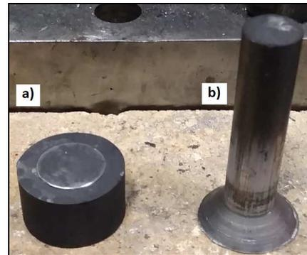
Fig. 3. Component assembly (a) and extruded bimetallic composite (b)
