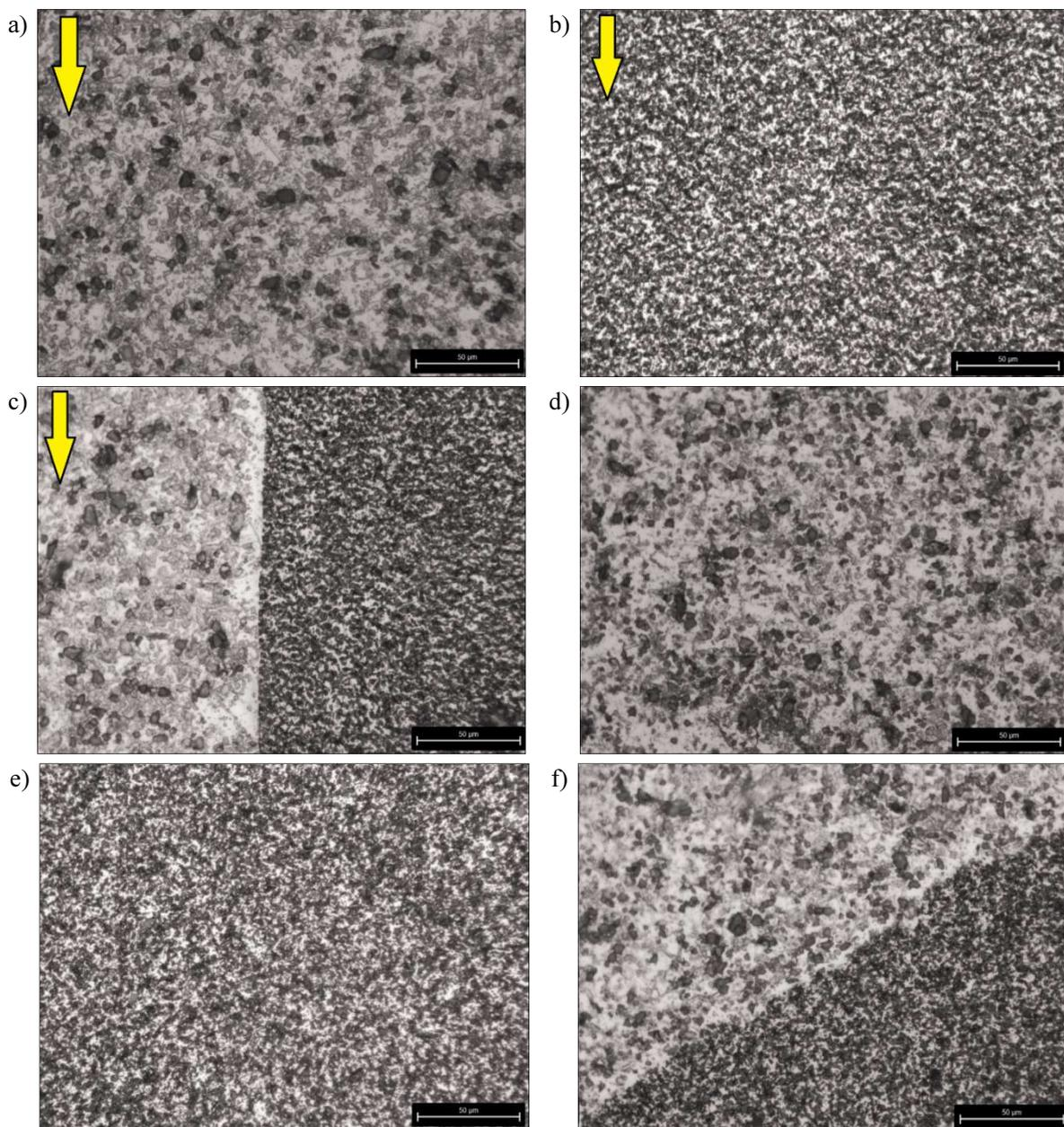
Fig. 6. Bimetallic composite obtained by extrusion at 480°C of component materials in Al17Si5Fe3Cu1.1Mg0.6Zr-cast aluminum rod sinter. Cross-sections: a, b, c longitudinal, d, e, f transverse. Zone: a, e sintered Al17Si5Fe3Cu1.1Mg0.6Zr, b, d sintered aluminum, c, e boundary between component materials. Etched
