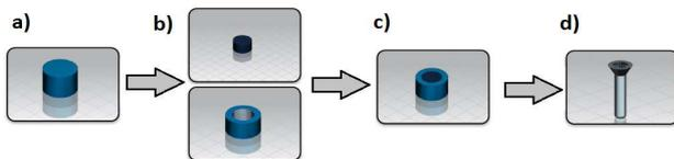
Fig. 2. Diagram of extrusion assembly fabrication: a), b) components, c) assembly, d) extruded bar
