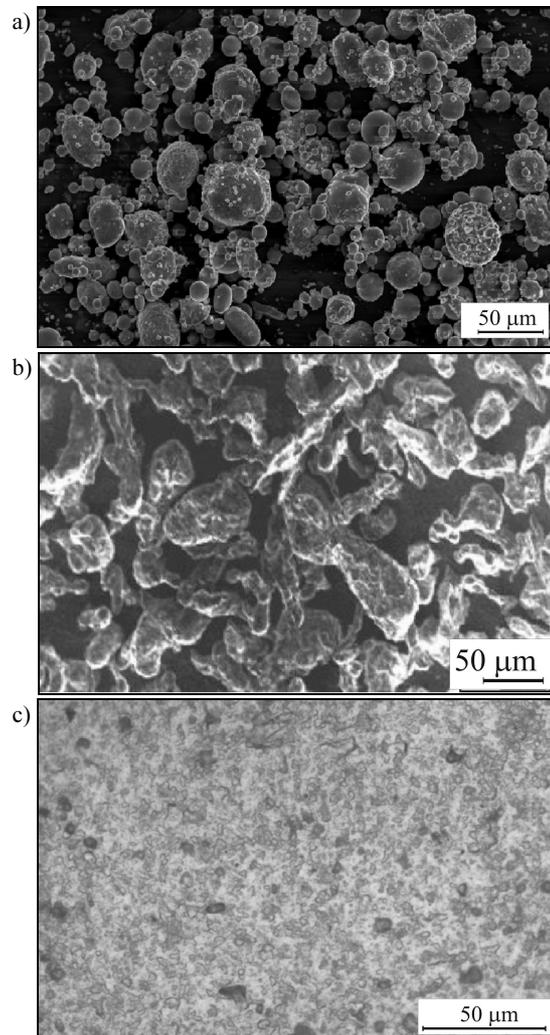
Fig. 1. a)  $\text{Al}_{17}\text{Si}_5\text{Fe}_3\text{Cu}_{2}\text{Mg}_{0.6}\text{Zr}$  powder, b) aluminum powder, c) aluminum rod microstructure
