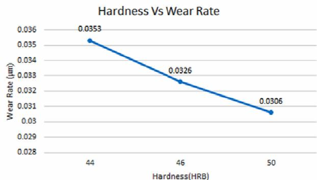
Fig. 7. Role of hardness in wear
