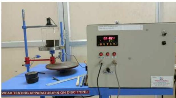
Fig. 2. Pin-on-disc equipment
