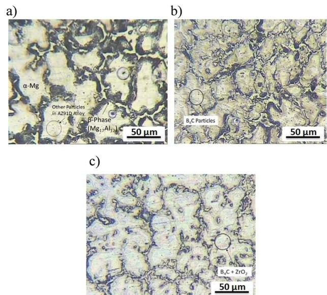
Fig. 4. Microstructure of: a) AZ91D, b) AZ91D+3% B<sub>4</sub>C, c) AZ91D+2% ZrO<sub>2</sub> + 3% B<sub>4</sub>C (recorded at 200 $\times$  magnification)
