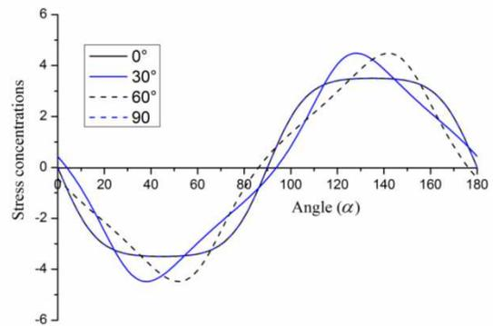
Fig. 4. Stress concentrations  $\sigma_\alpha/S$  versus  $\alpha$  for four layered woven glass-epoxy composite
