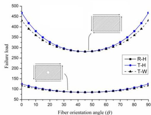
Fig. 9. Effect of notch presence and fiber orientation angles on failure load of glass-epoxy laminates
