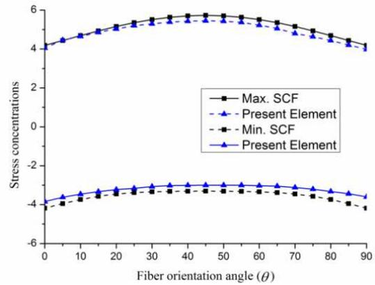
Fig. 7. Stress concentration factors  $\sigma_a/S$  versus fiber orientation angles for glass-epoxy plates
