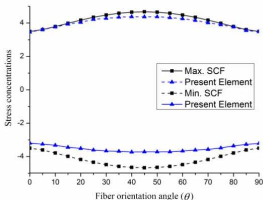
Fig. 6. Stress concentration factors  $\sigma_a/S$  versus fiber orientation angles for woven glass-epoxy plates
