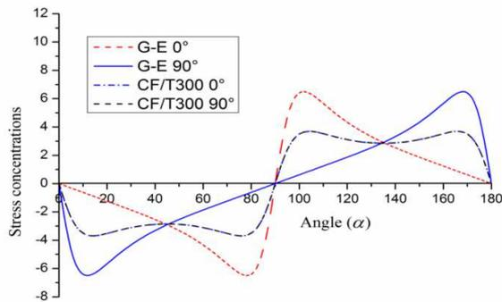
Fig. 3. Stress concentrations  $\sigma_\alpha/S$  versus  $\alpha$  for two laminate composites (graphite-epoxy and CF/T300)
