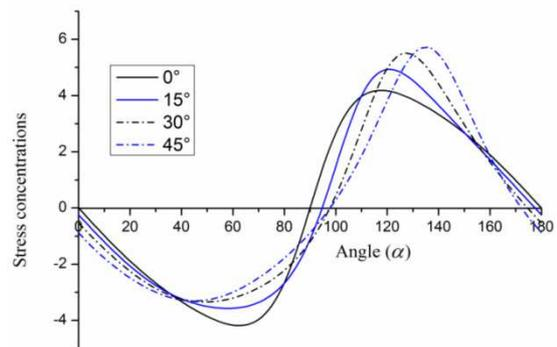
Fig. 5. Stress concentrations  $\sigma_\alpha/S$  versus  $\alpha$  for four layered glass/epoxy composite
