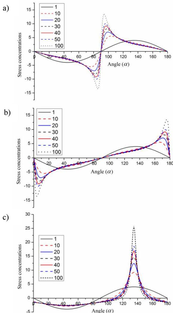
Fig. 8. Stress concentration  $\sigma_\alpha/S$  versus  $\alpha$  for different modulus ratio  $E_1/E_2$  and fiber orientation: a)  $\theta = 0^\circ$ , b)  $\theta = 90^\circ$ , c)  $\theta = 45^\circ$
