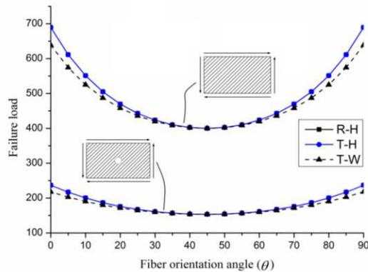
Fig. 10. Effect of notch presence and fiber orientation angles on failure load of graphite-epoxy laminates
