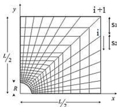
Fig. 1. Finite elements mesh of quarter of plate
