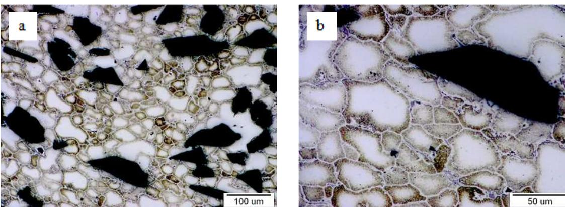
Fig. 10. Microstructure of Al<sub>4</sub>Cu + 10 wt.% SiC composite
