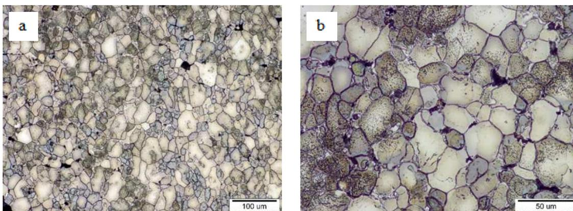
Fig. 8. Microstructure of as-sintered Al<sub>4</sub>Cu
