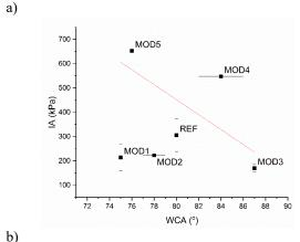
Fig. 3. Ice adhesion values as a function of (a) Ra; (b) WCA
