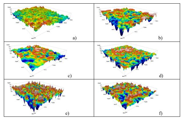
Fig. 1. 3D visualization of fabricated surfaces by means of profilometer: a) REF, b) MOD1, c) MOD2, d) MOD3, e) MOD4, f) MOD5
