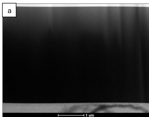
Fig. 2. TEM/ BF low (a) and high magnification (b) micrographs of cross-section of FeCrNi/a-C:H coating
