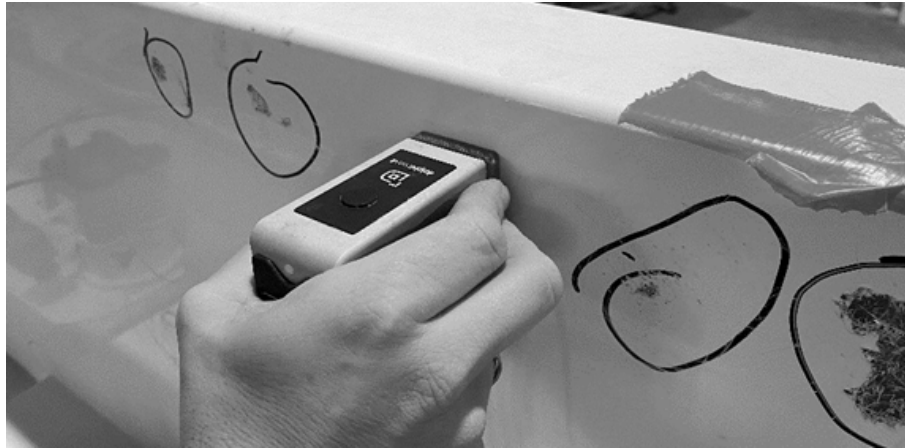
Fig. 6. Inspected area. Left and right side of probe are areas with visually detected blisters
