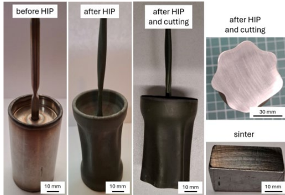
Fig. 4. Capsule before and after HIP process, Fe sinter
