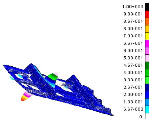
Fig. 4. Buckling analysis for optimized panel
