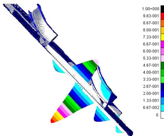
Fig. 5. Buckling analysis for optimized panel (particular)
