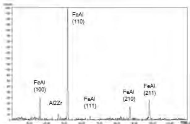
Fig. 4. Results of X-ray phase analysis of alloy 2% vol.  $\text{Al}_2\text{O}_3$ +Fe40Al
