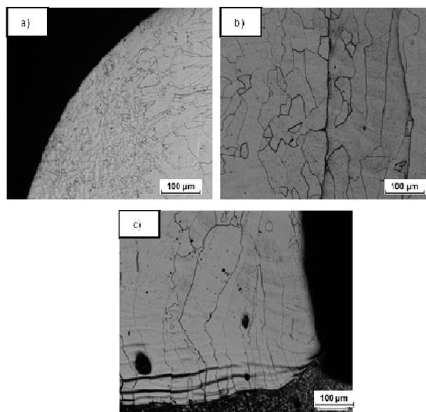
Fig. 3. Microstructure of alloy Fe40Al 2% vol. and Al<sub>2</sub>O<sub>3</sub>: a) at edges, b) in volume, c) base
