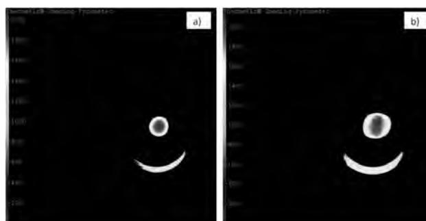
Fig. 8. Temperature distribution in lake of molten metal alloy: a) without nanoceramics, b) with nanoceramics [11]
