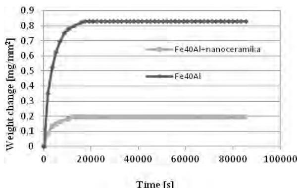
Fig. 5. Thermogravimetric curves (800°C, 24 h) for matrix alloy phase nanoceramics Fe40Al without addition of  $\text{Al}_2\text{O}_3$  and addition of 2% vol. nanoceramics  $\text{Al}_2\text{O}_3$
