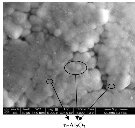
Fig. 1. Morphology and composition of Fe40Al+0.05%Zr +50 ppm. B+ +2% vol.  $\text{Al}_2\text{O}_3$  powder after low-energy milling for 10 min. at 200 rpm
