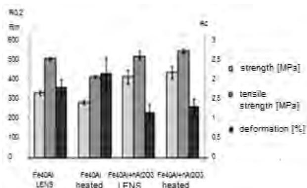
Fig. 7. Summary of parameter values obtained during static tensile test
