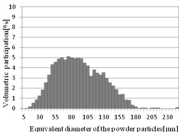
Fig. 2. Histogram of particle size distribution of Fe40Al+0.05% Zr+50 ppm B with 2% vol. Al<sub>2</sub>O<sub>3</sub> after milling at 200 rpm for 10 min. during analysis of IPS U
