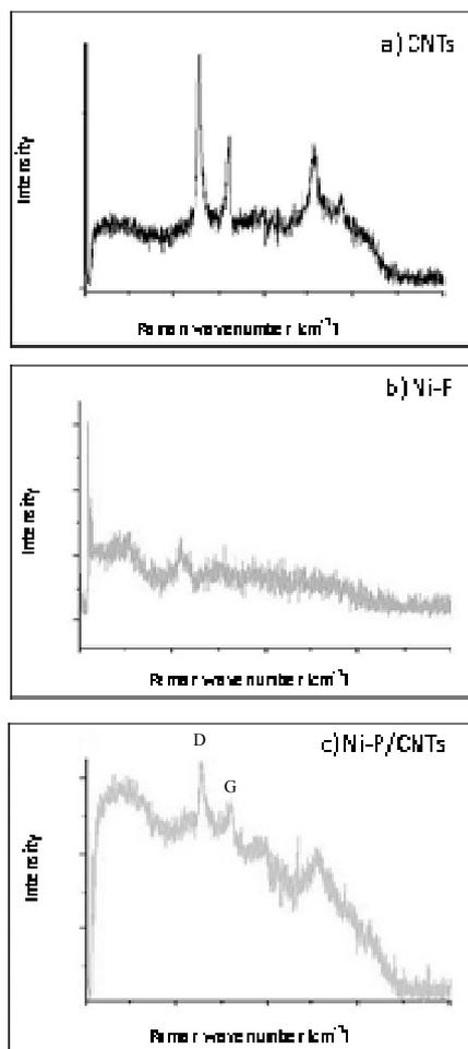
Fig. 6. Raman plots of: a) CNTs, b) Ni-P layer, c) Ni-P/CNT composite layer
