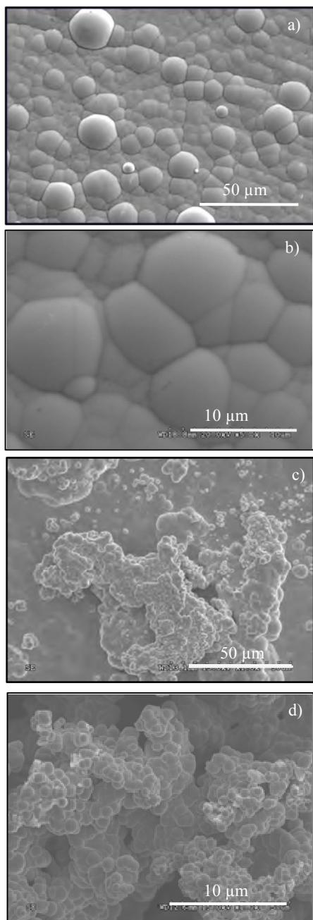
Fig. 3. Morphology of: a) and b) Ni-P layers, c) and d) Ni-P/CNTs composite layers
