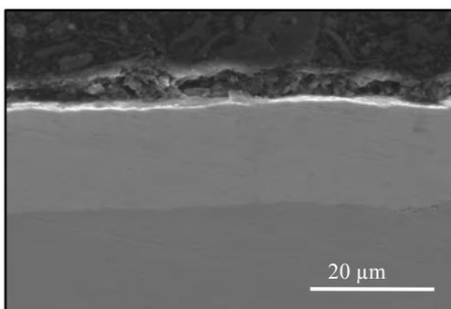
Fig. 4. Cross-section morphology of Ni-P/CNTs composite layers
