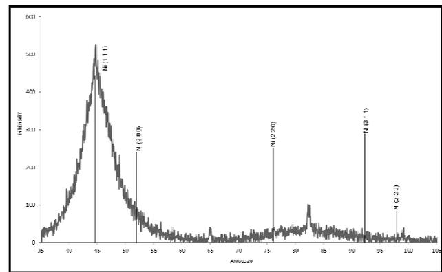
Fig. 2. Diffraction patterns of Ni-P layers
