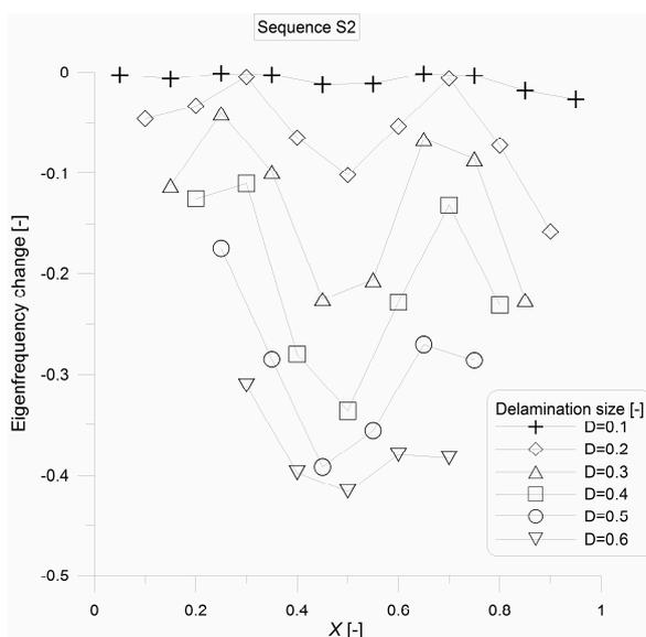
Fig. 6. Relative drop of third eigenfrequency ( $f_3$ ) of composite cantilever beam
