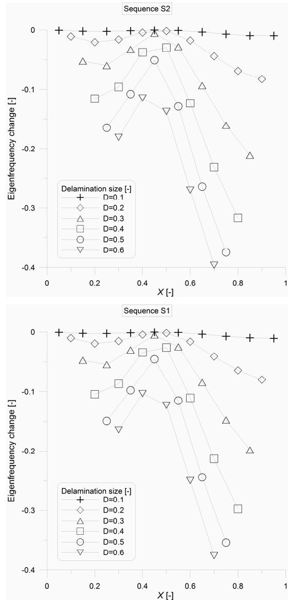
Fig. 5. Relative drop of second eigenfrequency ( $f_2$ ) of composite cantilever beam
