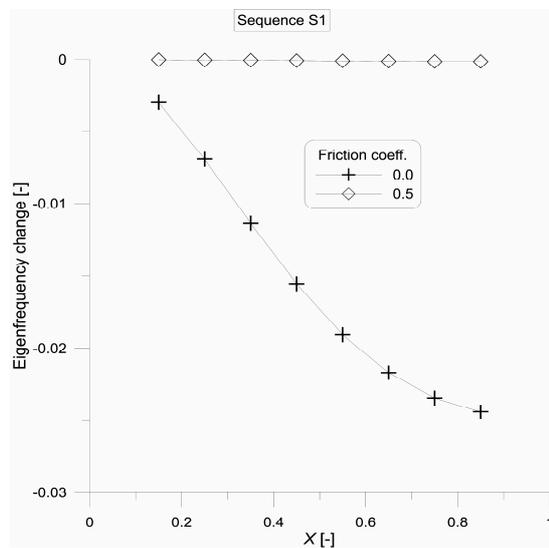
Fig. 7. Relative drop of first eigenfrequency ( $f_1$ ) of composite cantilever beam when friction is taken into account
