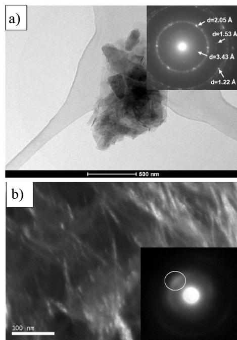
Fig. 1. TEM micrograph of N006 graphene platelet and electron diffraction pattern shown in insert (a); TEM micrograph of FLRGO platelets taken using dark field diffused reflection marked by white circle shown in insert (b)
