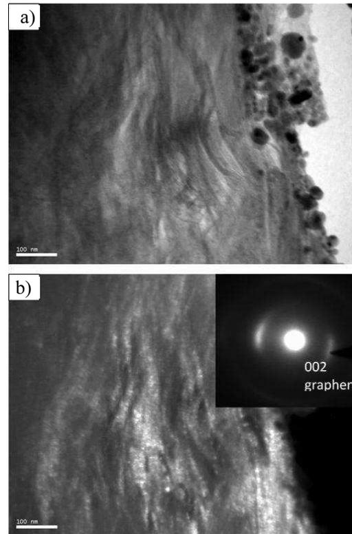
Fig. 7. TEM micrograph in bright field of silver based composite with 2% FLRGO graphene platelets (a); Dark field micrograph showing bright lamellar graphene taken using basal plane diffused 002 graphene reflection visible in diffraction pattern shown as insert (b)
