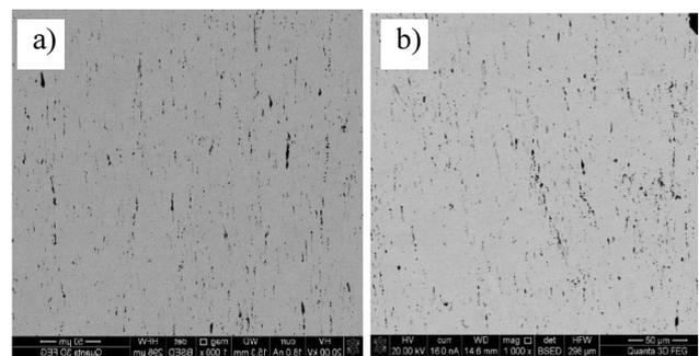
Fig. 8. SEM micrographs of hot pressed and extruded Ag-matrix composite containing (a) 1% FLRGO graphene platelets and (b) 2% FLRGO graphene platelets
