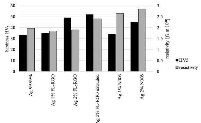
Fig. 5. Changes in hardness and electrical resistivity of hot pressed silver matrix composites containing either 1 or 2 wt.% N006 or FLRGO graphene platelets. Resistivity is only slightly higher in comparison with that of silver ( $1.59 \cdot 10^{-8} \text{ W m}$ )
