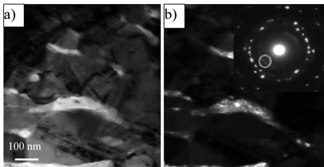
Fig. 6. TEM micrograph of silver based composite containing 2% N006 graphene (a); Dark field image taken using diffused reflection of elongated graphene platelet marked with white circle in electron diffraction pattern shown in insert (b)
