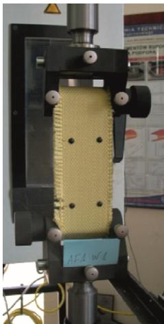
Fig. 2. AF1 fabric sample mounted in capstan grips; test at temperature  $T_1$
