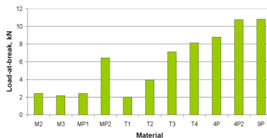
Fig. 1. Original load-at-break of materials used in the study
