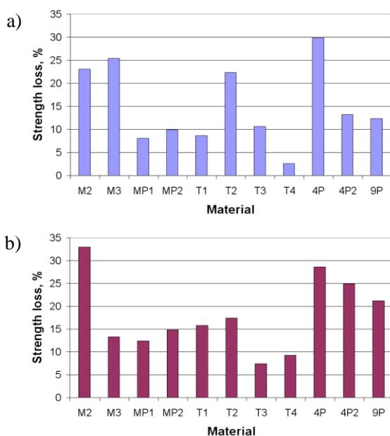
Fig. 4. Strength loss: a) after 5.4 J impact, b) after 7.35 J impact
