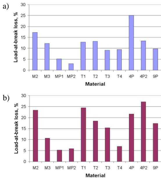
Fig. 3. Load-at-break loss: a) after 5.4 J impact, b) after 7.35 J impact
