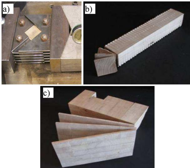
Fig. 1. Production process for end grain boards: a) densification device, b) densified squared timber, c) glued block and sliced end grain board
