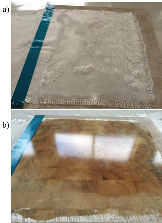
Fig. 2. Balsa core with glass fabric and powder resin (a) and finished composite structure (b)
