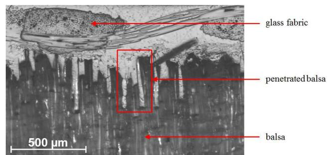
Fig. 3. Microscopic image of glass-balsa sandwich
