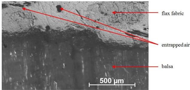
Fig. 4. Microscopic image of flax-balsa sandwich
