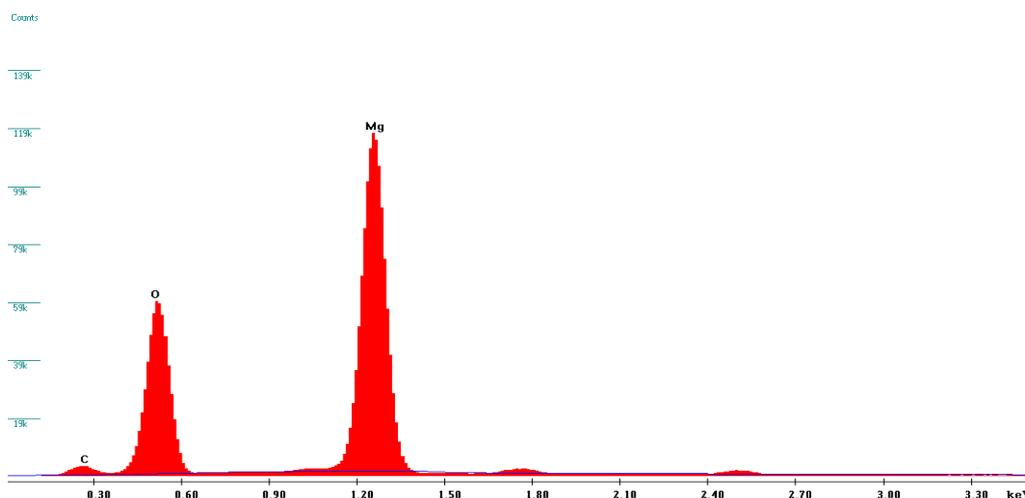
Fig. 2. EDS analysis of chemical composition of powder formed as result of thermal decomposition of basic magnesium carbonate
