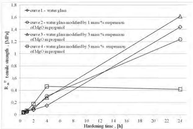
Fig. 3.  $R_m^U$  tensile strength of loose moulding sands with water glass, unmodified and modified. Hardening conditions: temperature  $t_{ot} = 23.5^\circ\text{C}$ , moisture content  $W_w - 39\%$
