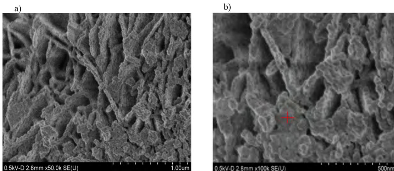
Fig. 1. Magnesium oxide (MgO) formed by thermal decomposition (a, b)
