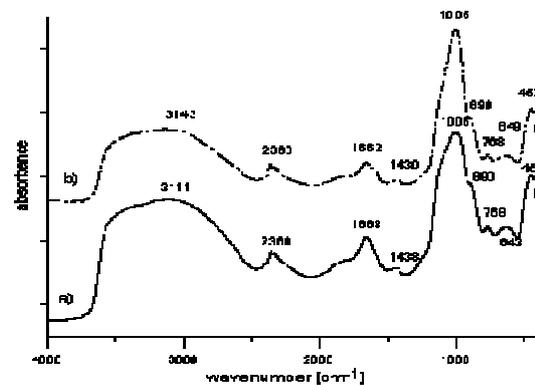
Fig. 6. Absorption spectra of: a) unmodified water glass, and b) water glass modified after 24 hours of hardening
