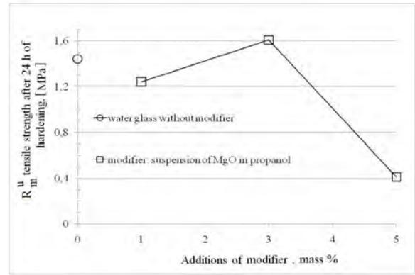
Fig. 4. Effect of modifier content on  $R_m^U$  tensile strength of loose moulding sands with modified water glass. Hardening conditions: time - 24 h, temperature  $t_{ot} = 23.5^\circ\text{C}$ , moisture content  $W_w - 39\%$
