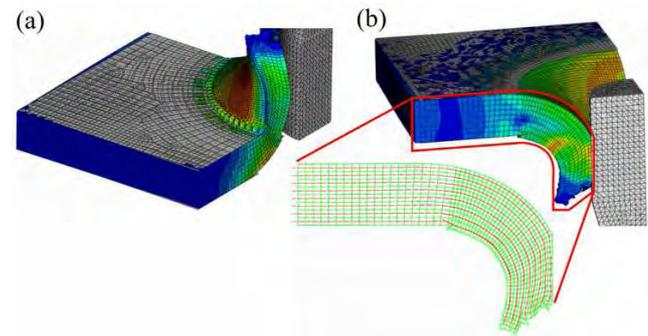
Fig. 6. Deformation of pure matrix indentation: (a) die-sided and (b) pin-sided with material texture in neck area representing probable fiber orientation
