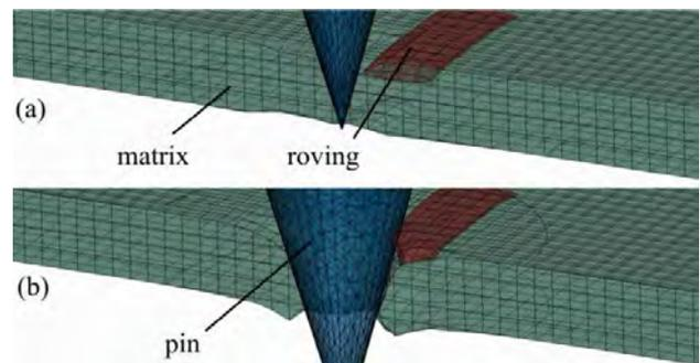
Fig. 7. Deformation of CEL analysis at two different stages: (a) before matrix split and (b) split matrix elements affect roving deformation
