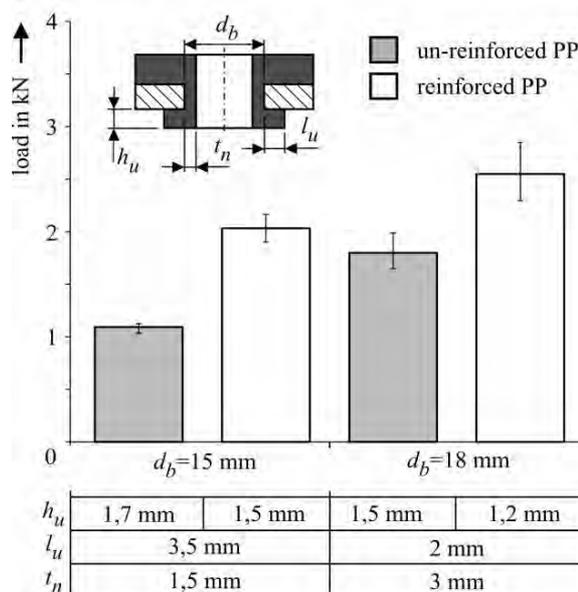
Fig. 4. Dependence of varying main joint dimensions on load bearing capacity of thermoclinching joints with both un-reinforced and reinforced thermoplastic joining partners
