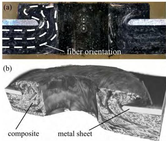
Fig. 5. Analyses of thermoclinched joint micro-structure by (a) micrograph analysis and (b) computed tomography
