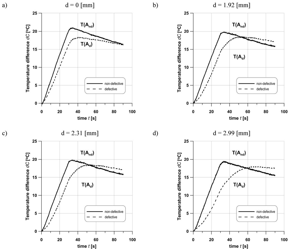
Fig. 7. Evolution in time of temperature difference  $dC$  for various loading conditions in defective and non-defective areas
