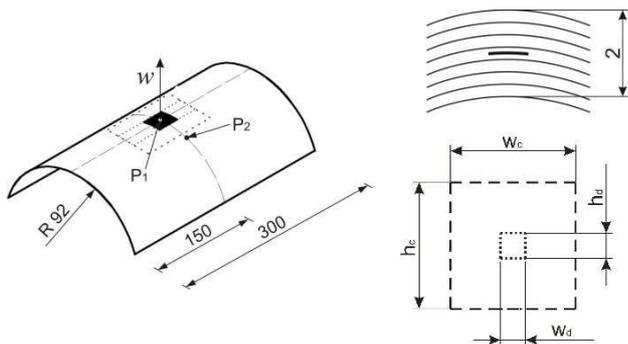
Fig. 4. Geometry of investigated specimens
