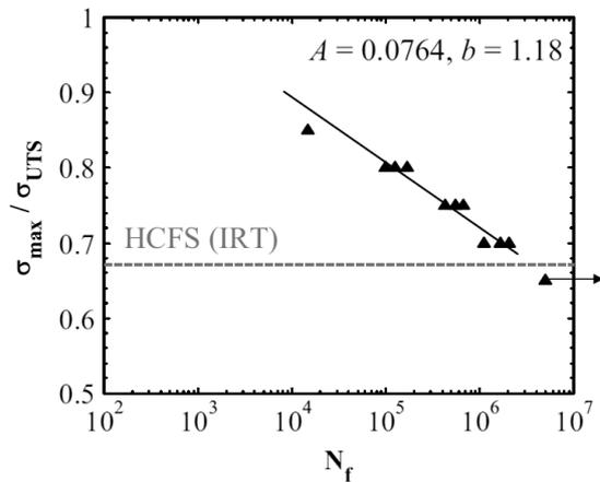
Fig. 1. Example of fatigue S-N experimental data for woven carbon fabric/epoxy composites with high cycle fatigue strengths (HCFS) obtained by IRT technique marked [26]
