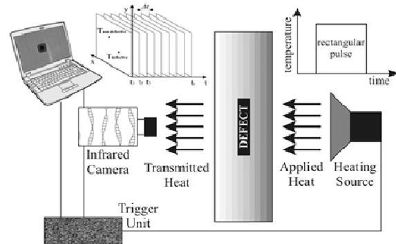
Fig. 2. Principle of pulsed infrared thermography
