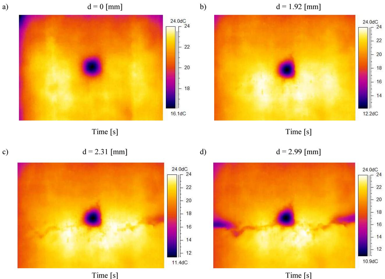
Fig. 6. Thermograms of cylindrical panel subjected to compression
