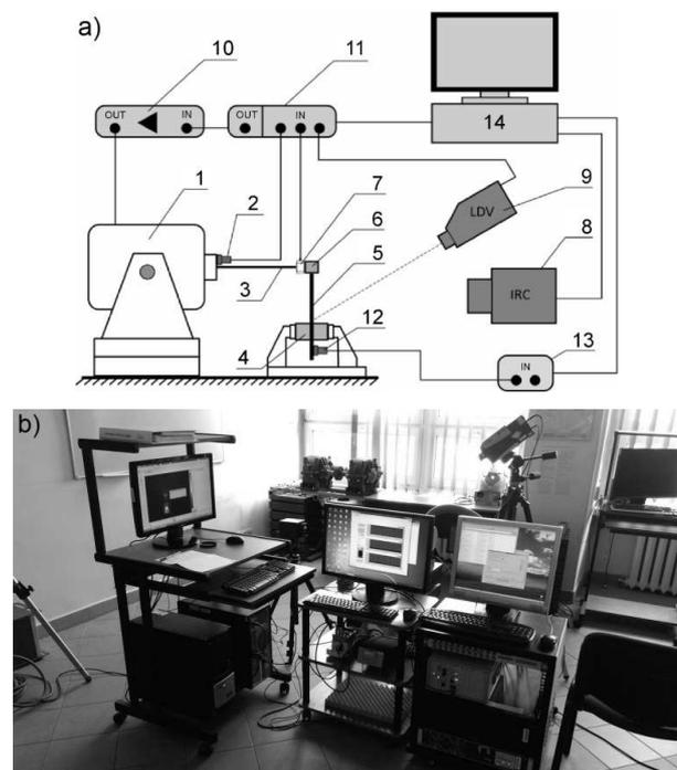
Fig. 1. Experimental test rig for performing fatigue tests: a) diagram, b) photograph
