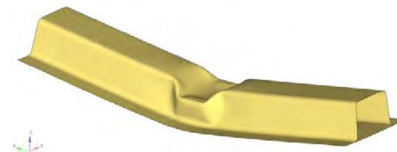
Fig. 9. Virtual deformation of validation segment, corresponding to crosshead displacement of  $s = 200$  mm
