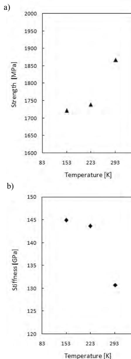
Fig. 1. Results of: a) tensile strength and b) stiffness of M12/35%/UD134/AS7/300 unidirectional specimen as a function of temperature
