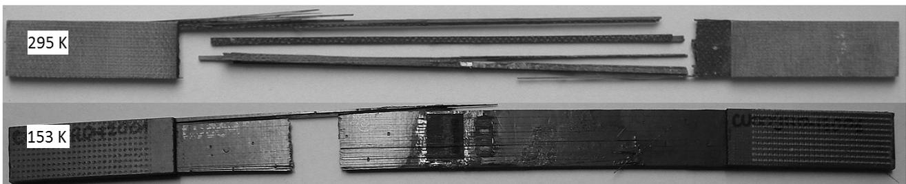
Fig. 3. Failure types of specimens destroyed in tensile tests at 295 and 153 K
