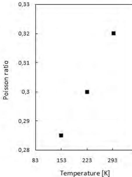
Fig. 2. Poisson ratio of M12/35%/UD134/AS7/300 unidirectional specimen as function of temperature
