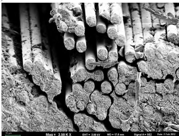
Fig. 4. SEM image of fracture surface morphology of samples tested (a) at RT, (b) at 153 K
