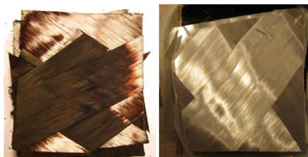
Fig. 4. Examples of specimens with carbon and glass (hybrid) fibers after calcination
