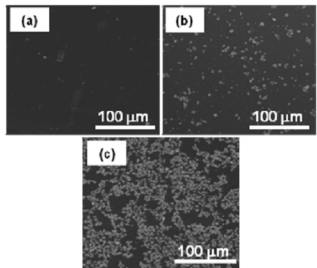
Fig. 3. SEM image after incubation in UHQ water solution of pure PGLA (a), composite surface of (b) PGLA/1.5 wt.% Ag and (c) PGLA/3 wt.% Ag
