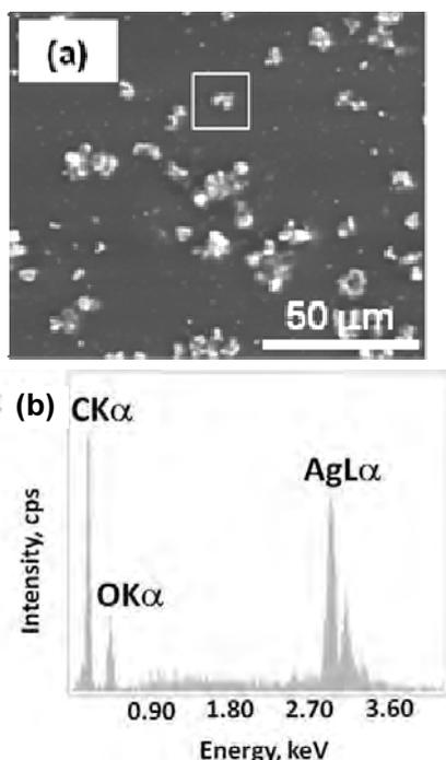
Fig. 4. SEM image (a) and EDS analysis in selected area (b) of PGLA/3 wt.% Ag after incubation in UHQ water solution
