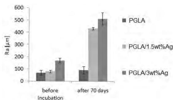
Fig. 6. Roughness of pure PGLA and PGLA/Ag composite samples before and after incubation in water solution
