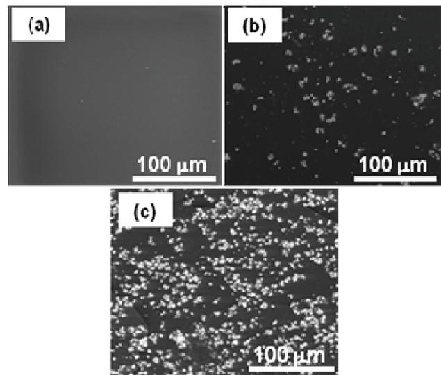
Fig. 2. SEM image of pure PGLA (a), composite surface of (b) PGLA/1.5 wt.% Ag and (c) PGLA/3 wt.% Ag
