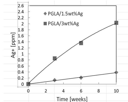
Fig. 8.  $\text{Ag}^+$  ions release during 10 weeks of sample immersion in UHQ water
