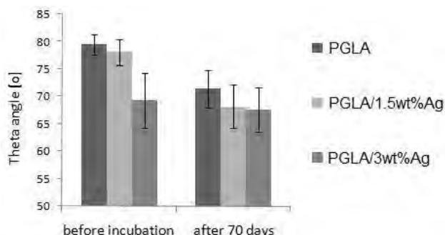
Fig. 5. Contact angle of pure PGLA and PGLA/Ag composite samples before and after incubation in water solution
