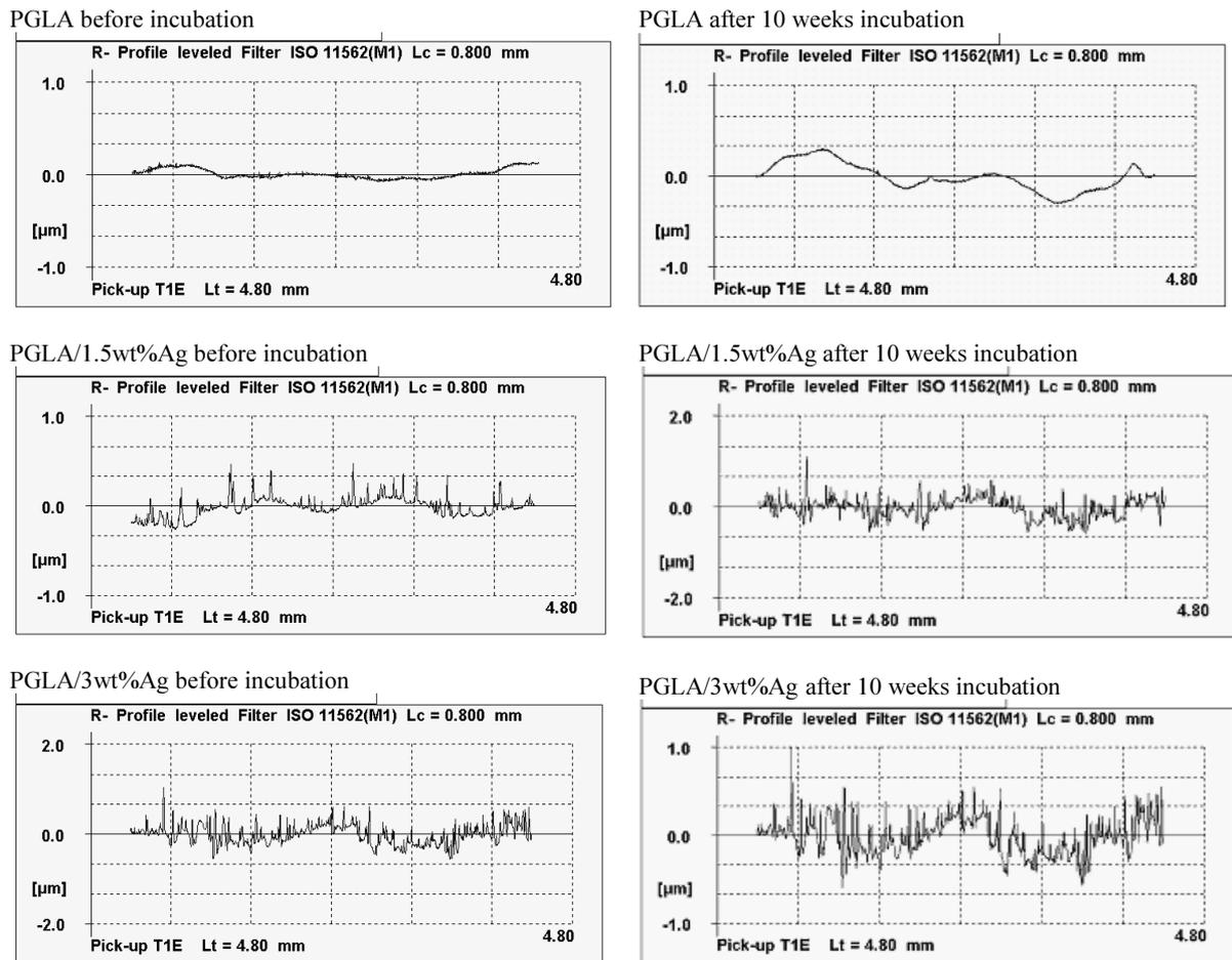
Fig. 7. Profile diagrams of pure PGLA and PGLA/Ag composites before and after 10 weeks incubation in water solution
