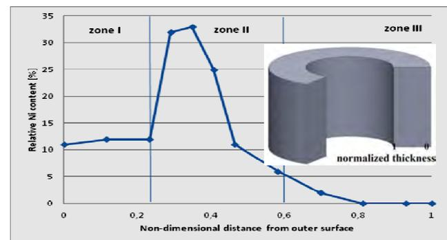
Fig. 6. Changes in sample metallic phase content from outer zone to inner zone
