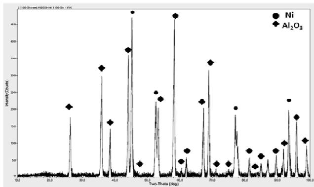
Fig. 3. XRD pattern of  $\text{Al}_2\text{O}_3$ -Ni composites
