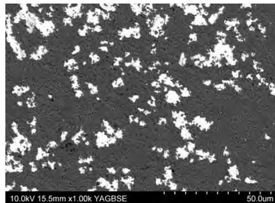
Fig. 5. Microstructures of specimens fabricated by centrifugal slip casting
