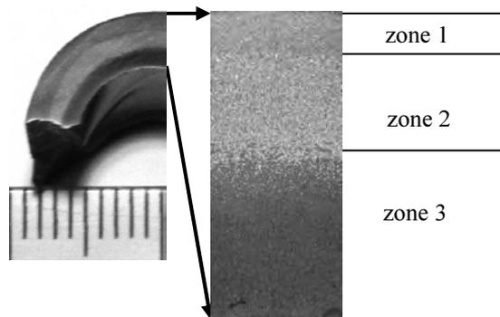
Fig. 4. Fragment of sintered composite sample cross-section fabricated by centrifugal slip casting in horizontal rotation axis, additionally marked zones I, II, III
