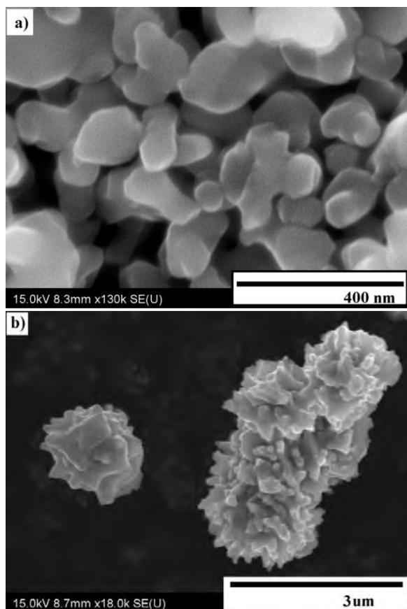
Fig. 1. SEM images of morphology of starting powders: a)  $\alpha$ -Al<sub>2</sub>O<sub>3</sub> powder, b) nickel powder
