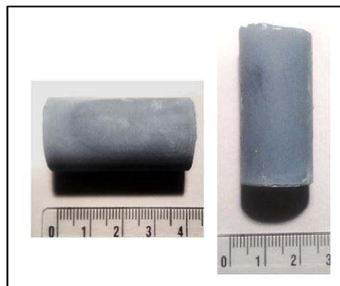
Fig. 2. Views of composites samples before sintering
